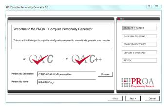
On the first page of the personality generator, ensure that QA·C is selected or QA·C++ if you are using QA·C++ and programming in C++. (Do not use QA·C++ for C source.)
