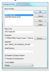
The next step is to configure QA·C to analyse a single C file. On the IAR EWARM IDE select the "Tools" menu as above and click on "Configure Tools" and the "New" in the tools dialogue.
