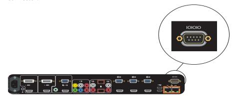
Use a DB-9 to DB-9 cable such as the Straight-Through Serial Cable on page 37 to connect to the RS-232 interface. The pinouts for this type of cable are listed in the following table:
