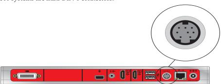
Use an 8-pin mini-DIN to DB-9 cable such as the Polycom RealPresence Group Series Serial cable on page 36 to connect to the RS-232 interface. The pinouts for this type of cable are listed in the following table:
