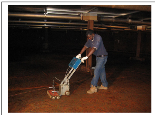
One type of MFL machine for floor scanning. Note: Internal floating roof.
