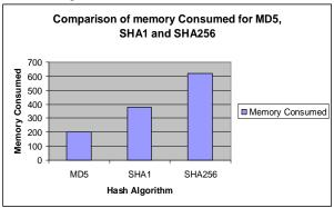
Fig. 7: Memory consumed for different hash algorithm
