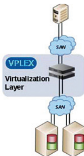
Figure 2: Storage access from VPLEX virtualization layer
