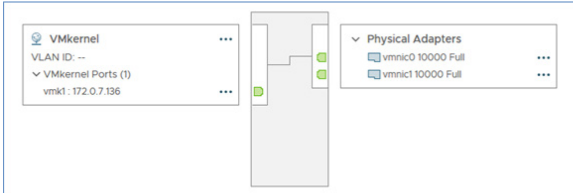
Figure 5 - vSwitch With 2 Physical Ports
