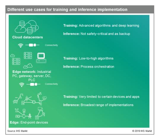
The graphic also points to the wired or wireless connectivity that links up edge end-points to the edge network and the edge network to the cloud. 5G will play an increasing important role here. IHS Markit expects that 5G will be integrated into several IoT gateway products before the end of 2019 to provide enhanced downlink and uplink bandwidth for commercial and mobile applications.
