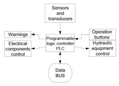
Fig. 2. Hardware structure of the data acquisition and control system of a designed test stand
