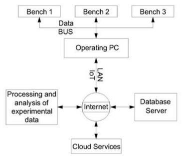
Fig. 3. Hardware structure of the computer system
