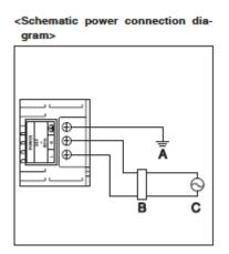
A. Earth B. Earth leakage breaker C. Power supply 24VAC 60 Hz
