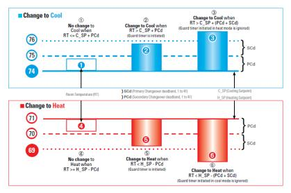
Figure 13. Cool/Heat Changeover Logic
