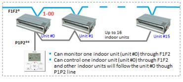
Figure 6. Assigning One Group Address to a Remote Controller Group
