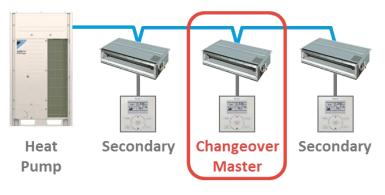
Figure 8. Heat Pump System
