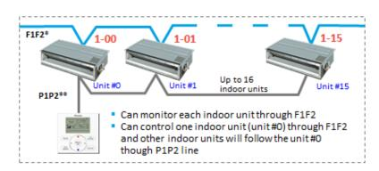
4. Assigning a group address to each indoor unit in a remote controller group:
