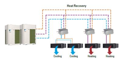
Figure 3. Heat Recovery System
