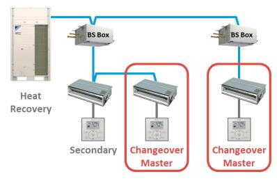
Figure 9. Heat Recovery System
