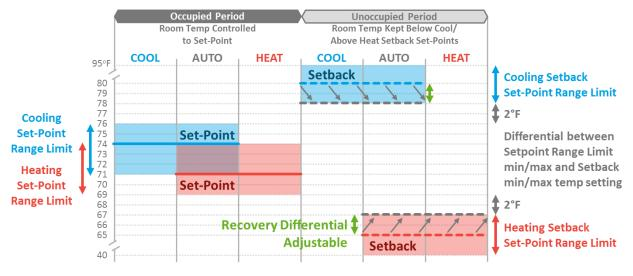
Figure 10. Relationship between Setpoints, Setback, and Setpoint Range Limitation
