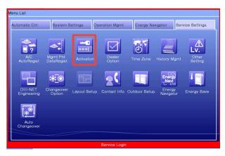
2. On the Activation Setup page, click the Add button to open the keyboard dialog box, and enter the activation key for the *iTM BACnet* Server Gateway option.
