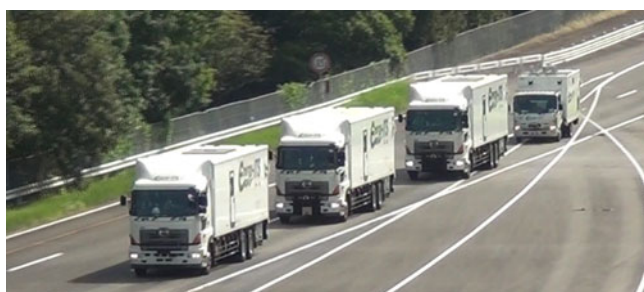
Fig. 1. The automated platoon of 3 heavy trucks and a light truck.
