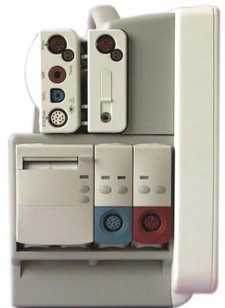
Side view of MP40/MP50 with MMS and MMS extension (top), and plug-in recorder module and two measurement modules below
