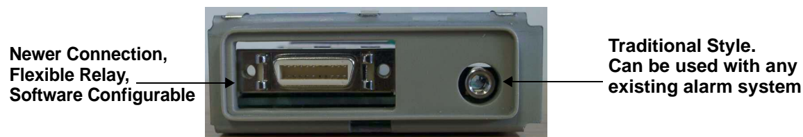
Figure 29 Flexible Nurse Call Relay Connections at Monitor
