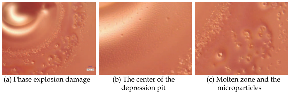
Fig. 2.8. Damage morphology induced by phase explosion (15kHz)
