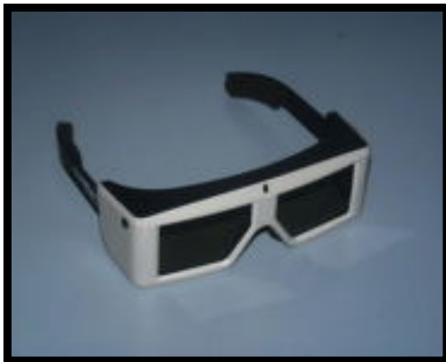
Shutter glasses: active device, frame sync, higher frame rates (120Hz okay)
