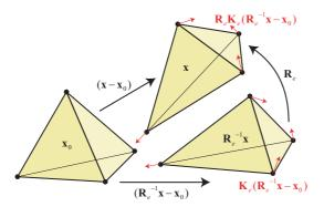
Figure 2: To compute the elastic forces acting at the vertices of a tetrahedron, its deformed coordinates  $\mathbf{x}$  are rotated back to an unrotated frame  $\mathbf{R}_e^{-1}\mathbf{x}$ . There the displacements  $\mathbf{R}_e^{-1}\mathbf{x} - \mathbf{x}_0$  are multiplied with the stiffness matrix yielding the forces  $\mathbf{K}_e(\mathbf{R}_e^{-1}\mathbf{x} - \mathbf{x}_0)$  that are finally rotated back to the frame of the deformed tetrahedron by multiplying them with  $\mathbf{R}_e$ .
