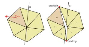
Figure 4: Planar sketch of a vertex split in 3-d. To fracture a tetrahedron, an adjacent vertex v is chosen. Plane  $\alpha$  is placed perpendicular to the maximum stress component  $\sigma_{\max}$  through v. Then v is split into  $v_+$  and  $v_-$ . Tetrahedra adjacent to v that lie on the positive side of  $\alpha$  are linked to  $v_+$ , the others to  $v_-$ .
