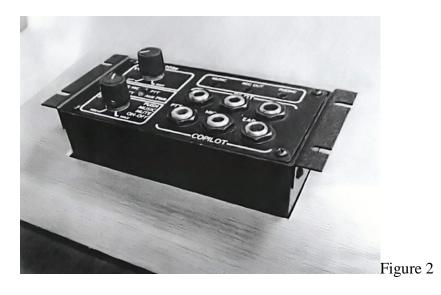
(The 205e with the mounting brackets installed.)
