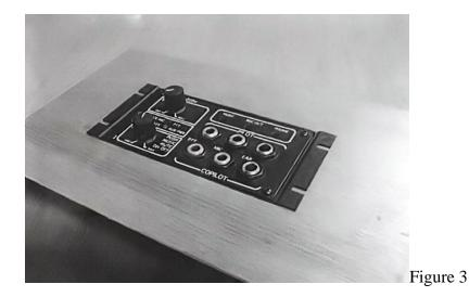
Push the intercom back into the hole, and use the bracket slots as a template to mark where to drill holes for the mounting screws. The slots in the brackets are intended for 6-32 screws. You can use nuts behind the panel to secure the screws, or use a smaller drill bit and thread the panel itself. In either case, use Blue LocTite or other suitable thread locker to make sure the screws cannot loosen from vibration.
