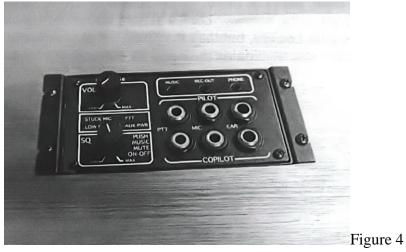
**To install with brackets behind the panel:** Cut the mounting hole 2.525" tall and 4.565" long. With the brackets behind the panel instead of in front, they will not aid in hiding any imperfections in the cut, so the ends of the mounting hole will have to be cut as precisely as the top and bottom. For the most exact fit, make the hole slightly smaller and file as necessary. **Be careful not to get any shavings or filings into the intercom.**
