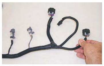
148. Remove the black tape and split loom from the MAF connector and wires. Pull the connector and wires back the point where the coil pack connector branch is located.
