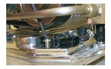
85. Install the intake manifold gaskets supplied into the recesses on the supercharger manifold face. Ensure that the gaskets are fully seated.
