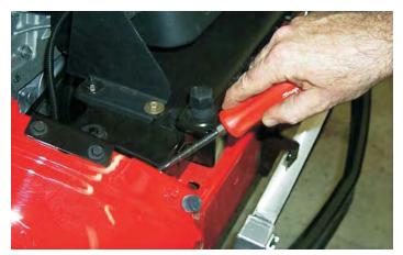
130. After pushing the molded foam block, pull it out from the engine compartment. The foam block will not be reused.
