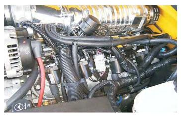
164. Route the new MAF branch forward to MAF and plug in the connector. Secure the branch as necessary with the tie straps supplied to keep it away from the belt and moving parts.
