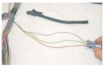
154. Install the new MAP harness to the Orange/black, Green and Gray wires using the crimp/shrink connectors supplied. The new harness wires are all white, so care must be take so the new white wires are in the same positions as the colored wires on the original connector. Strip about ¼" of insulation from the ends of all the wires. Crimp the connectors on and shrink the insulation so that it contracts around the wires completely.
