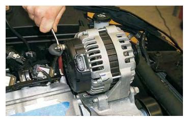
49. Disconnect the positive (+) battery cable from the back of the alternator with a 10mm wrench. Use a 15mm socket wrench remove the two bolts holding the alternator to the alternator bracket and then remove the alternator.
