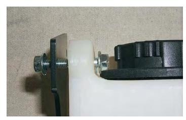
118. Remove the bolt and washer that secures the front mounting foot of the radiator coolant tank. Insert the lower mounting tab of the intercooler reservoir under the foot of the coolant tank and reinstall the bolt and washer. Tighten the bolt securely with a 10mm socket wrench.
