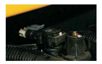
33. Disconnect the evaporative purge solenoid EVAP connector located on the top of the driver (left) side fuel rail, by raising the black plastic retaining clip and then pull free the connector itself.
