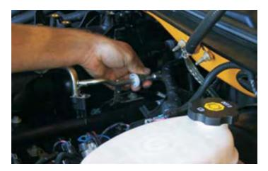
40. Using a 8mm socket wrench remove the ten intake manifold bolts.
