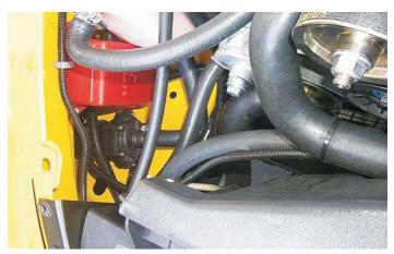
168. Lift the cover off the FUSE/RELAY CENTER and set aside for re-installation.
