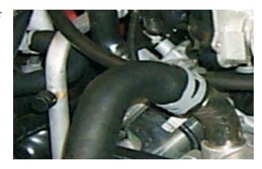
72. The original water pump outlet tube will need to be replaced. Remove the outlet by cutting it off. Use a suitable hacksaw and cut it off approximately 1" above the water pump casting.
