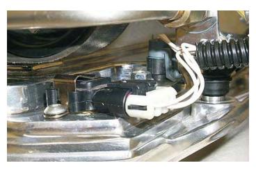
163. On the driver side of the engine, plug in the Alternator, Injector #1, Coil pack, injector #3, #5, #7, and EVAP connectors.
