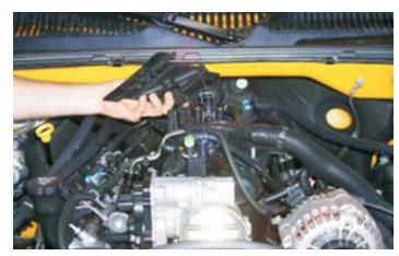
30. Disconnect the eight fuel injector connections by gently pulling up on the gray plastic release trigger on the connector and then pulling firmly on the connector itself. Disconnect the coil pack connector and then the four wire harness clips that secure the harness to the right side of the engine.
