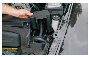
6. There are three computer connectors, Grey, Black and Blue. Remove the connectors by first removing the Red locking key, then pushing in on the Black cover and pushing the Grey latch down.
