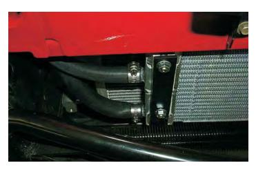
139. Route the hose up from the lower opening and across the back side of the air filter cover to the remaining barb on the coolant manifold. Cut the intercooler hose to length and secure both ends with a #10 clamp. Note: The rotation of the MAF and the location of the MAF electrical connection.
