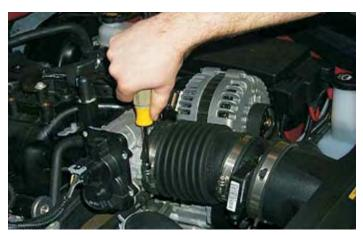
20. Unplug the Mass Air Flow meter (MAF) connector by pulling out the gray release trigger and the squeezing the connector.
