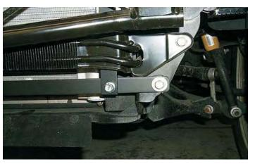
128. Here is the mounting bolt on the right side of the vehicle. Note: The heat exchanger barbs must be pointing to this side.
