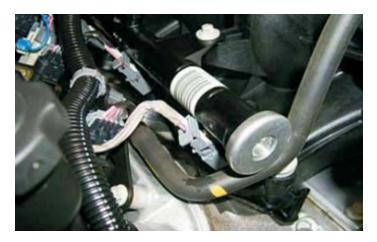
31. Disconnect Electric Throttle Control (ETC) connector from the throttle body by removing the gray plastic locking tab first, then squeeze and pull free the ETC connector itself.
