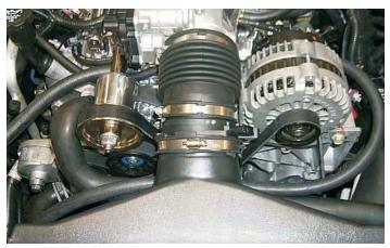
140. Route the 1/4" hose from the coolant reservoir to the barb on the steam pipe. Cut the hose to length and secure this end with the new #6 clamp supplied.
