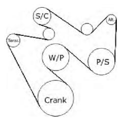
144. With the drive belt installed, rotate the water pump outlet and upper radiator hose out of the way of the supercharger drive pulley. Lock the water outlet into position by tightening the outlet retainer bolt securely with a 12mm wrench.
