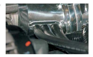
109. Install the new check valve into the brake booster.
