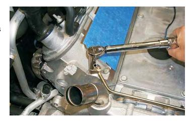
56. Using the supplied 3/8" hose, connect a 15" length to the PCV valve as shown and lay the other end of the hose off to the drivers side, out of the way. (To be connected in a later step.)
