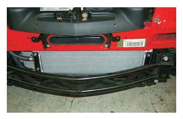
127. Using a 15mm wrench, remove the mounting bolts on both sides of the vehicle that are located below the power steering cooler bracket. Slide the heat exchanger up into position and then attach its mounting bracket with the original mounting bolts.
