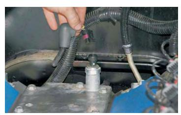
58. Remove the Oil Pressure Transmitter with a 28mm socket wrench.
