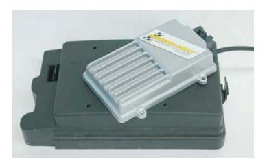
183. Using a 10mm socket wrench, attach the Magnavolt module to the top of the Fuse/Relay Center cover with the nuts and bolts supplied. Replace the inner and top covers on the FUSE/RELAY center.
