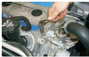
45. Remove the vent pipe assembly. (Make sure that the O-ring gaskets did not stick to the cylinder heads, if so remove them.)
