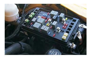
181. Remove the bolt that secures the large RED battery cable to the terminal at the Fuse/Relay center with a 7mm socket wrench. Attach the RED fused power supply wires of the relay and Magnavolt harness by passing the bolt through the ring connectors. Tighten the bolt securely.
