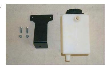
117. Assemble the reservoir to the mounting bracket using the two 6 x 20mm bolts and nuts supplied. Position the bracket so that the lower mounting tab is pointing away from the reservoir. Tighten securely with a 10mm socket wrench.
