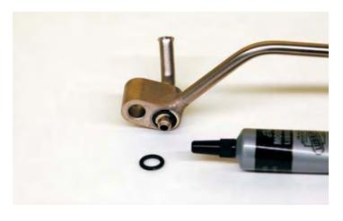
55. Using the stock bolts removed in step 45 install the new coolant vent pipe supplied. Ensure that the O-ring gaskets are installed correctly. Torque the bolts with a torque wrench and 10mm socket to 106 lb-in.
