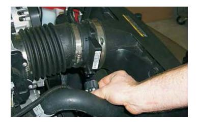
21. Remove the two plastic push-lock rivets from the air filter apron. Do this by gently prying the center of the rivet up with a straight blade screwdriver and then removing the rivets completely.
