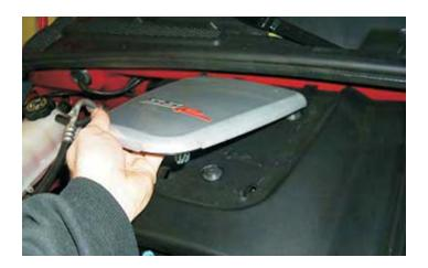
17. Remove the engine cover's four fasteners with a 8mm socket wrench.
