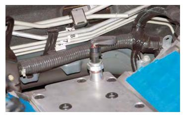
65. Using a 13mm wrench remove the bolt securing the attachment clip for the fuel line.
