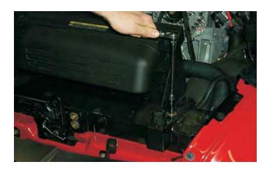
25. Remove the air filter assembly complete and then separate the MAF and bellows from the air filter cover.
