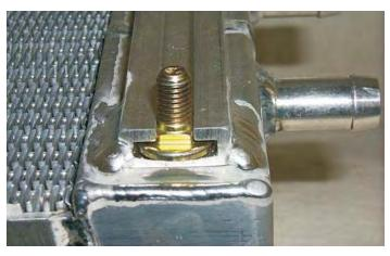
122. Align the bolts with the holes in the vertical mounting brackets.
