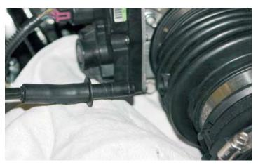
28. Open the large electrical harness retainer clip, then using a 10mm socket wrench remove the bolts holding the plastic wire harness retainer to the intake manifold
