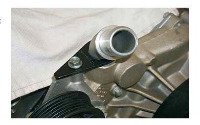
81. Install the upper radiator hose and clamp onto the new water pump outlet.
