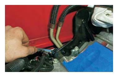
66. Remove the steel bracket on the rear of the left cylinder head with a 15mm wrench, the bracket will not be reused.
