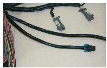
158. Remove about 5" of the large 1-1/4" split loom from the main trunk of the harness. Cover the exposed portions of the main harness with the new 3/4" loom starting from the left side injector branches to the right side coil branch. Tape and secure the new branches as necessary.
