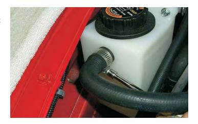
137. Connect the short end of the 90 degree "Elbow" hose to the pump inlet and the long end to the bottom (outlet) barb of the reservoir. Secure both ends with #10 clamps. Connect the remaining length of hose to the outlet barb of the pump and route it through the opening that was uncovered when you removed the molded foam block.
