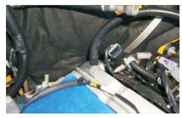
57. Remove the rubber cover and then the electrical connector from the Oil Pressure Transmitter.
