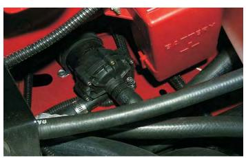
134. From underneath the vehicle on the right side locate the elongated hole. Approximately 1" back from the hole drill a 1/4" hole to mount the pump. Place the mounting clamp around the pump body and then pass the new 6 x 20mm bolt through the pump mounting clamp and then through the hole. Secure the bolt with the new nut and tighten securely with a 10mm wrench.
