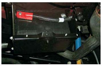
3. Locate the vehicles computer just below the windshield washer reservoir filler neck. Remove the two bracket bolts with a 10mm socket wrench.
