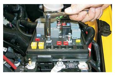
172. Remove the small positive battery cable from the bottom of the Fuse/Relay Center by un-clipping its connector with a small straight blade screwdriver.
