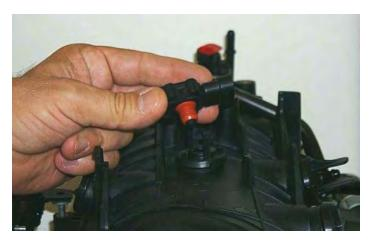
83. Put some lubricant on the MAP sensor seal and press the MAP sensor into the provided hole in the supercharger manifold as shown.
