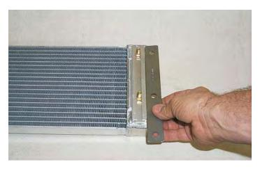
123. Torque the mounting nuts to 18 ft-lbs with a 13mm torque wrench.
