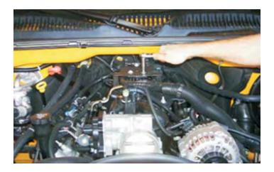
29. Using a 10mm socket wrench, remove the three bolts that fasten the cover support bracket from the top of the intake manifold.
