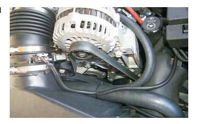
165. Here is the Intercooler Relay wiring and the Magnavolt module with its components.
