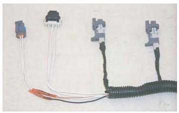
156. Locate the Purge solenoid connector branch on the main branch of the harness.
