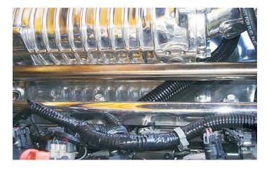
161. On the passenger of the engine, plug in the ETC, A/C, Coil pack and Injector #2, #4, #6, #8 connectors.
