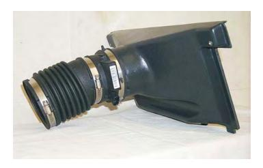
115. Reinstall the bellows to the throttle body and then re-attach the air filter box and its apron to the vehicle.
