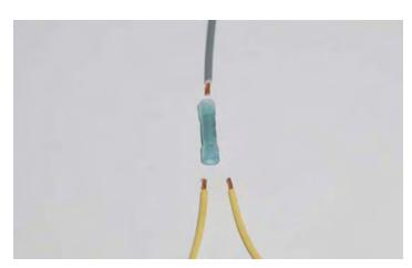
175. Using a heat gun or a blow-dryer set on high, shrink the plastic covering of the connector until the clear sealant from the inside of the connector can be seen oozing out from under the plastic covering. Crimping the connector alone is not enough to insure a permanent connection; you must shrink the plastic covering!
