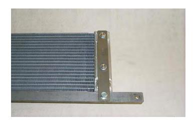
125. Here is the completed heat exchanger ready for installation. Note: The heat exchanger barbs and long end of the cross member are on the right side.
