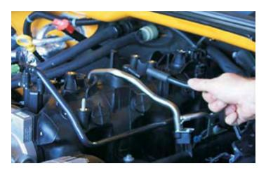
38. Remove the power brake hose and check valve from the brake booster.
