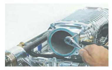
94. Mount the throttle body using the original nuts and bolts. Torque to 106 in-lbs.
