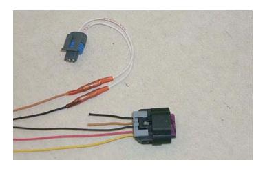
151. Continue to remove the black tape and split loom from the main branch of the harness to the point where the remaining MAF connector and wires emerge from the harness at the point just above the branch for the drivers side injectors.
