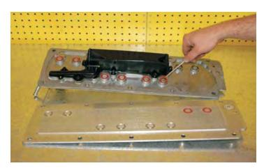
62. Install the new engine valley cover and flathead bolts supplied with a 5mm Allen socket and torque the bolts to 18 lb-ft. Insert the six O-rings in the recesses in the new valley cover.
