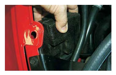
131. Removing the molded foam block creates a opening between the radiator and the fender well for the intercooler coolant lines to pass. The line from the pump to the heat exchanger and from the heat exchanger to the coolant manifold will pass through this opening.
