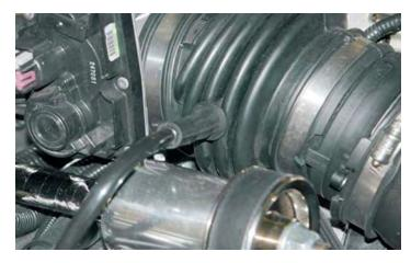
102. Locate the vent tube previously removed from the tube from the vehicle.
