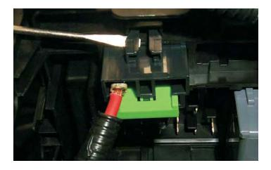
173. Unscrewing the harness connector anchor bolt will allow the large white plug to be removed from the bottom of the Fuse/Relay Center. Locate the GREY wire in the bundle and cut it approximately 1-1/2" from the connector.
