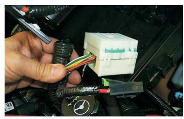
174. Install a crimp/shrink connector by cutting the grey wire and stripping a ¼" of insulation off each end. Into one end of the connector, insert the end of the GREY wire from the large white plug. Into the remaining end insert the end of the YELLOW wire from the intercooler relay and the YELLOW wire from the Magnavolt harness and crimp it securely.
