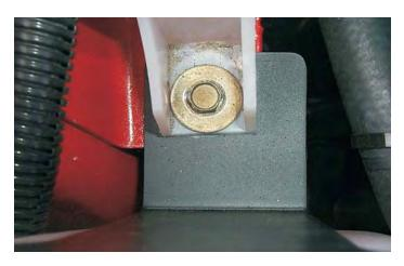
119. Here is the installed intercooler reservoir and bracket on the vehicle.
