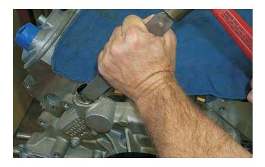
74. Use a pair of pliers to pull the collapsed stub straight up and out. Do not twist the stub as you pull it out, as this will scratch the outlet bore of the water pump casting.
