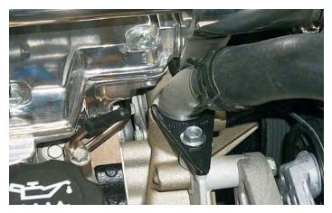
82. Remove the stock MAP sensor from the stock intake manifold by pulling back on the two tabs and lifting the sensor out. Ensure that the orange MAP sensor seal is not damaged, as it will be used.
