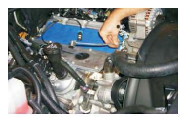
46. Using a 15mm tensioner wrench or breaker bar, remove the stock serpentine belt from the vehicle. The belt will not be reused.
