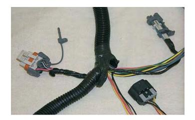
149. Locate the Tan and the Black wires that are next to each other on the connector, these are the Intake Air Temperature (IAT) circuit. Approximately 1" back from the MAF connector cut these wires.
