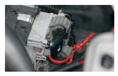
7. The computer connectors can be removed when the latch is pushed down and the red tail of the latch is visible on the end of the connector.
