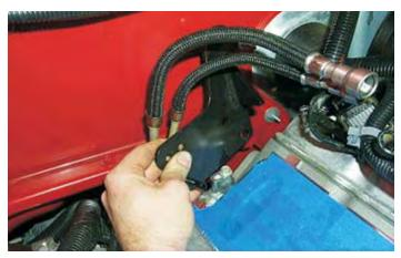
67. Remove the two bolts securing the firewall seam cover from the firewall with a 10mm socket wrench.
