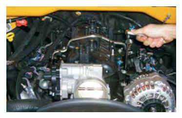
41. Carefully remove the intake manifold assembly and set aside.
