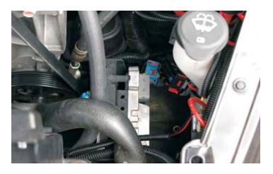
9. Note: If your vehicle has a automatic transmission, you will also need to remove the transmission control computer located on the back side of the mounting bracket.
