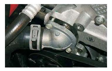
27. Remove the PCV vent pipe on the throttle body inlet bellows.
