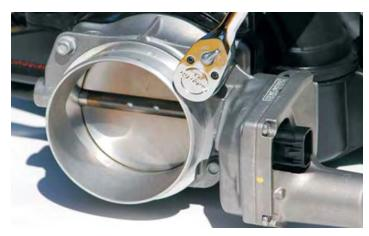
90. Next, using a #5 internal Torx socket remove the mounting studs from the stock intake manifold.
