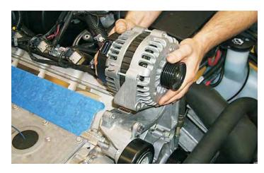
50. It will be necessary to make clearance on the alternator mount casting for the new manifold to fit properly. The new manifold should not touch the alternator mount. These modifications can be easily done with the mount in place.
