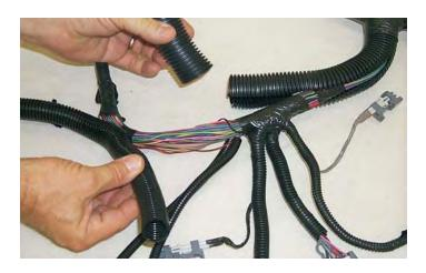
159. Re-secure the harness to the mounting clamp near the drivers side coil pack.
