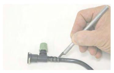
104. Assemble a new EVAP hose using the fittings and a 10" long piece of the 5/16" vapor hose with the #4 hose clamps supplied.
