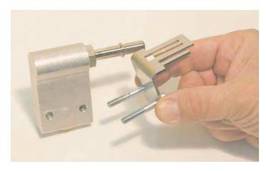
87. Using some of the lubricant supplied, install the O-ring into the recess on the fuel rail. Install the fuel manifold and bracket onto the fuel rail. Take care not to pinch the O-ring.
