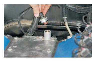
59. Remove the engine valley cover and gasket by removing the ten bolts with a ratchet and 13mm socket.
