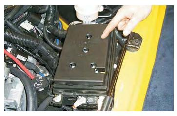
170. Lift the body of the FUSE /RELAY CENTER up off its base by unfastening the five snaps located along its bottom edge where it meets the base.
