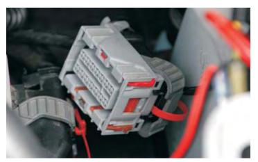
8. Release the computer module by lifting the two retaining hooks and lifting the computer out and up.
