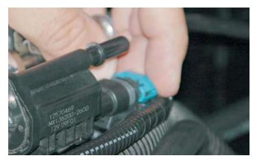
34. Disconnect the Air Conditioning (A/C) pressure connector from the pressure switch and from the clip on the cylinder head.
