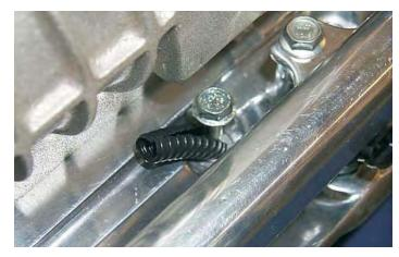
98. Torque all ten bolts that secure the manifold to the cylinder heads gradually and evenly to a torque of 89 lb-in. Use a 10mm socket and torque wrench.
