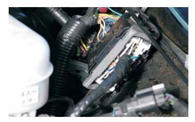
178. On the male end of the connection, locate the SOLID WHITE wire. This is the Engine Speed Signal (RPM) wire.
