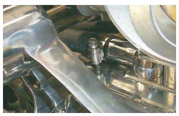
136. Route the hose to the top barb (inlet) on the reservoir. Secure the hose with a #10 clamp. Ensure that there are no kinks in any of the hose to restrict coolant flow.
