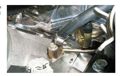
141. Install alternator on the stock bracket and torque the fasteners to 40 ft-lb.
