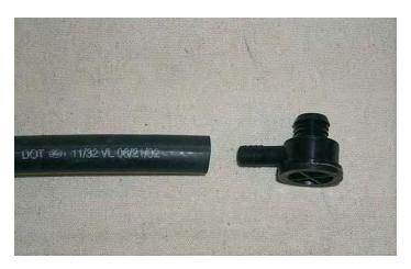
108. Connect the other end of the vacuum hose to the remaining barb on the side of the inlet manifold.
