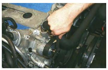
47. Using a 15mm socket wrench remove the three bolts holding the factory belt tensioner to the bracket and remove the tensioner.
