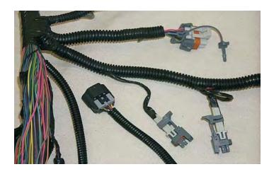
153. Locate the MAP connector on the harness. Remove the black tape and split loom from the MAP connector and wires. Viewing the connector from the top or clip side note the location and colors of the three wires on the connector, Orange/black left, Green center and Gray on the right. Approximately 1" behind the connector cut these three wires.
