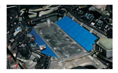
60. The gasket will be reused, the original valley cover and bolts will not. Inspect the gasket for any damage and then reinstall. Note: It will only fit correctly in one position.
