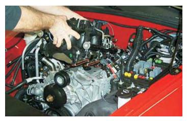
42. Using a vacuum cleaner, remove any dirt or debris from the intake port area. (Be careful not to get any dirt in the intake ports.) Note: 6.0L engines will not have the Knock sensor wells on the engine valley cover as shown.
