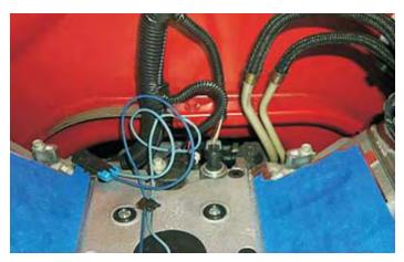
71. Remove the upper radiator hose at the upper water pump outlet.
