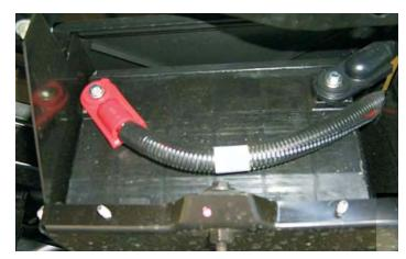
190. Replace the battery access panel and bolts. Secure them with a 10mm socket wrench.
