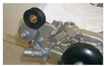
77. Install the two O-rings supplied into the grooves on the new water pump outlet.
