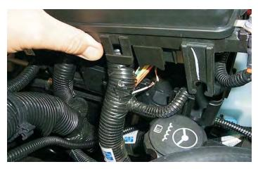
171. Unscrew the harness connector anchor bolt on the Fuse/Relay Center with a 7mm socket wrench. The bolt will become loose in the hole but cannot be removed.
