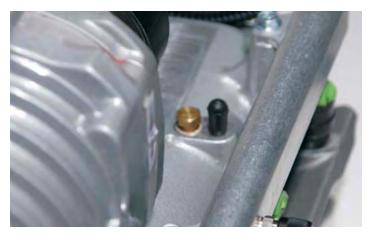
186. Using the hose supplied, connect one end of the hose to the pressure port and then route the other end to the Magnavolt module. Secure the hose out of the way of the rotating parts at the rear of the blower with the Ty-wraps supplied.
