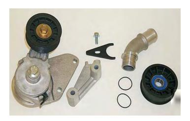
76. In the original tensioner location, mount the new outlet base with the new tensioner assembly on top of it. Use only the two long mounting bolts, the third shorter bolt will not be reused. Replace the factory idler pulley mounted on the alternator bracket with the new pulley supplied. Tighten the mounting bolts and with a 15mm socket and torque wrench to 40 lb-ft
