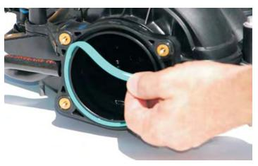
92. Install the throttle body O-ring into the inlet manifold groove on the supercharger.
