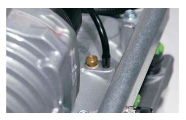
187. Connect the remaining end of the hose to the hose on the Magnavolt module using the hose connector supplied. Secure the hose out of the way with the Ty-wraps supplied.
