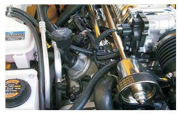
162. At the rear of the supercharger on the passenger side, plug in the new MAP and IAT connections.
