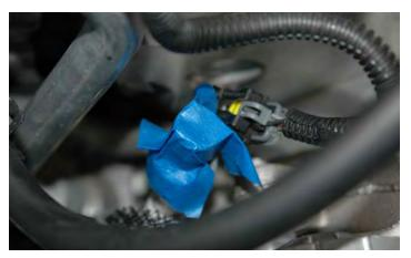
35. Lift the electrical harness from the top of the engine and set off to the drivers (left) side.
