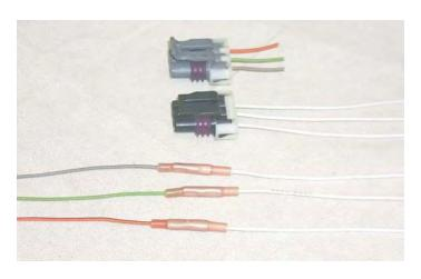
155. Group the IAT branch and MAP branches together and route them along the main branch to the #6 and #8 injector branch. Continue the IAT and MAP branches into the split loom of the right rear injector branch so that they exit the loom after the #8 injector connector. Cover the new branches with spilt loom and tape.
