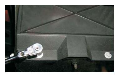
2. With a 8mm wrench disconnect the negative (-) battery cable and wrap the terminal end with electrical tape. Ensure that the cable is far enough away from the battery that it does not accidently touch the battery and make contact during the installation.
