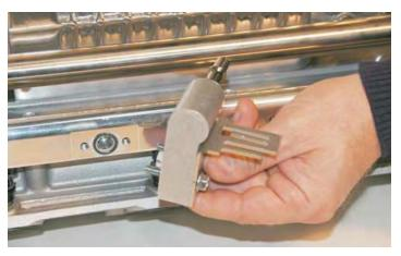
88. Torque the fuel manifold bolts to 106 in-lbs using a 10mm socket and torque wrench.
