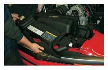
24. Remove the two remaining bolts securing the air filter with a 10mm socket wrench.
