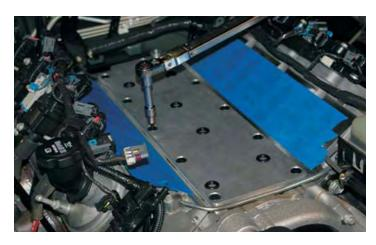
63. Install the Oil Pressure Transmitter in the new valley cover with a 28mm socket and torque it to 15 lb-ft.
