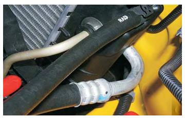
132. Here is the intercooler pump, mounting clamp, hardware, wiring and reservoir to pump hose.
