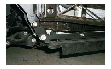
129. To create a space for the coolant lines to pass through the heat exchanger, you must remove the molded foam block located between the side of the radiator and the body. To remove the molded block, push it free with a straight blade screwdriver between the fender and the radiator support.
