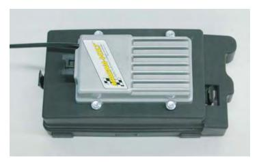
184. Insert the Magnavolt harness connector into the module until it locks into place.
