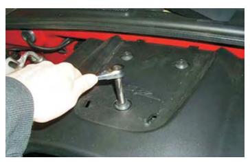
18. Remove the engine cover completely, as it and the SSR badge will not be reused.
