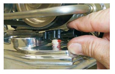
84. Using a 4mm Allen wrench, install the MAP sensor retaining clip with the provided 6mm button head screw as shown.
