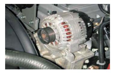
142. Re-attach the battery cable to the alternator terminal.
