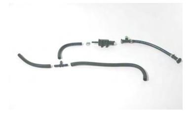
106. Install the PCV hose from the front of the "T" fitting on the middle barb of the inlet manifold.
