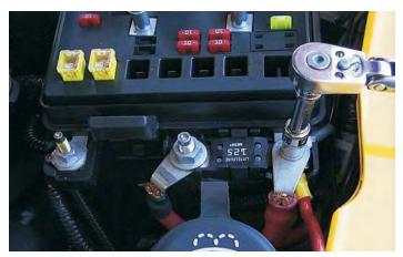
182. Start the Magnavolt installation by removing the cover to the Fuse/Relay Center. Using the Magnavolt uit as a template, mark and drill four 5/16"holes in the top of the cover.
