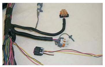
152. Cover the remaining MAF wires with the 1/4" split loom and tape to the point where the MAF wires meet the main branch of the harness.
