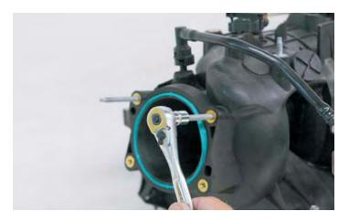
91. Remove the throttle body O-ring from the intake manifold.
