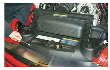
22. Remove the nuts and washers from each side of the air filter apron with a 10mm socket wrench.
