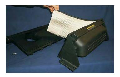
112. Assemble the air box with the new filter cover supplied.
