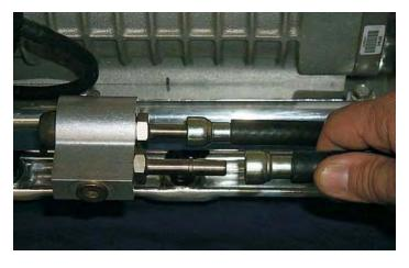
100. Remove the EVAP solenoid from the mounting bracket on the driver side fuel rail.
