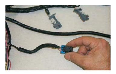
157. Remove the split loom and tape from the wires and pull the connector and wires back the point where the drivers coil pack branch is located. Cover the Purge branch with the new 1/4" loom supplied.
