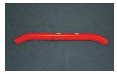
69. Cut the seam cover in two pieces with a suitable saw.
