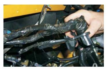
147. Locate the MAF connector on the wiring harness. The MAF connector is located at the front of the passenger side (right) branch that supplies the fuel injectors and ETC and AC.
