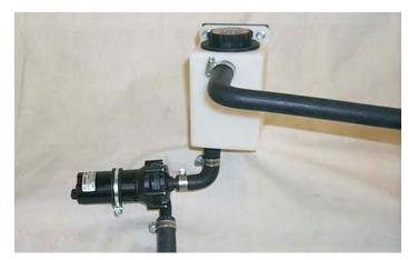
138. Route the hose to the bottom barb (inlet) on the heat exchanger. Cut the hose to length and secure both ends with a #10 clamp. Connect the remaining end of the hose to the upper barb of the heat exchanger and then back through the opening.
