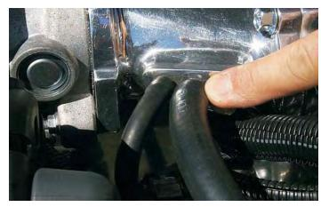
107. Insert the new vacuum check valve into the end of the new 11/32" Vacuum hose.
