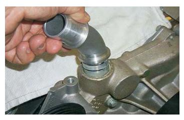
80. Install the outlet retainer and 8 x 20mm bolt into the tensioner base. Do not tighten the retainer bolt yet as final positioning will be done in a later step. Tighten the bolt finger tight for now.
