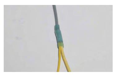
176. Connect the GREY wire from the Magnavolt harness to the remaining end of the Grey wire in the wiring harness with a Blue crimp/shrink connector.
