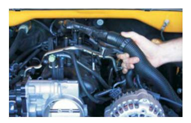
36. Disconnect the EVAP vent tube from the solenoid by squeezing the retainer, then release the tube from the solenoid located on the top of the fuel rail on the driver (left) side. Follow the same procedure on the other end of the vent tube at the firewall and remove the tube from the vehicle.
