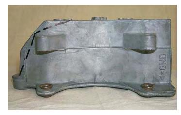
52. On the back surface of the alternator mount, remove the shaded area as shown.
