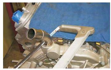
73. Remove the remaining stub of the outlet in the pump casting by collapsing it within itself. The object is to reduce the diameter of the stub by collapsing it not to cut it. Use a dull chisel or wide drift with a hammer to drive one side of the stub across and down to the other side. Take care not to damage or scratch the outlet bore of the water pump casting
