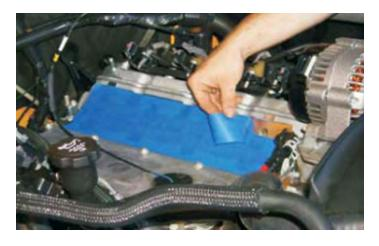
44. Using a 10mm socket wrench remove the two coolant vent pipe bolts.
