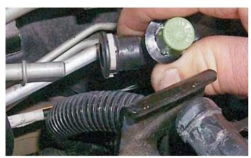
37. Remove the Positive Crankcase Vacuum (PCV) hose from the intake manifold on driver side.
