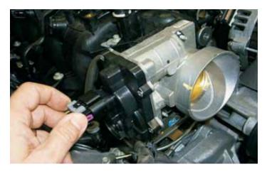
32. At the rear of the of the intake manifold disconnect the Manifold Absolute Pressure (MAP) sensor connector by gently raising the gray plastic retaining clip and then pull free the connector.
