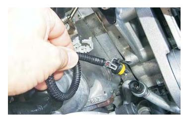
35. THIS STEP IS IMPORTANT! Cover the Air Conditioning (A/C) pressure switch with masking tape to protect it during the supercharger installation process.
