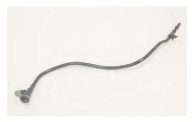
103. Using a sharp knife, cut the plastic tube at the ends to free the two EVAP fittings.
