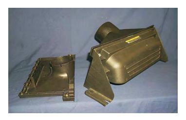
113. Secure the new filter cover with the original fasteners and a 10mm wrench.
