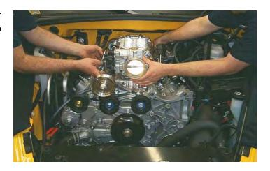
97. Remove the split-looms that support some of the manifold to cylinder head bolts. Start all ten bolts by hand to ensure proper alignment of the manifold.
