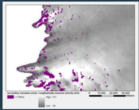
Areas of initial surface crevassing were prescribed where the calculated tensile stress exceeds the tensile strength of the ice (determined from crevasse locations on imagery).
