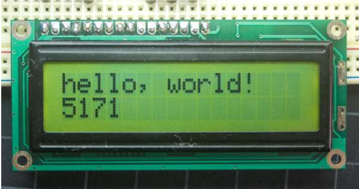
Figure 5: An LCD screen displaying text from example code
