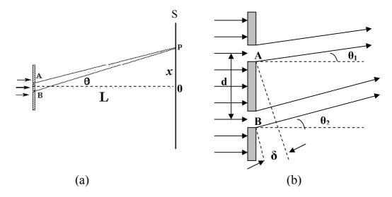
Fig. 3. Diffraction of the primary beam on the slits A and B produces interference pattern on the screen S behind the obstacle. INTERFERENCE & DIFFRACTION
