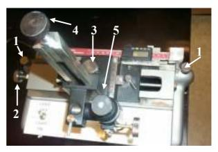
Fig.7. Microscope: 1 – screws for leveling the table; 2 and 3 – screws for adjusting the position of the tube in horizontal plane; 4 – screw for coarse vertical
