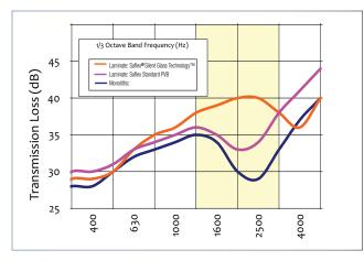
Figure 1: Sound Transmission Loss of Monolothic Glass, Laminated Glass with Saflex SilentGlass Technology and Saflex R series interlayer. Laminated glass configuration: 3mm glass/0.76mm interlayer/3mm (1/8in./0.030 in Saflex interlayer/1/8 in) glass.
