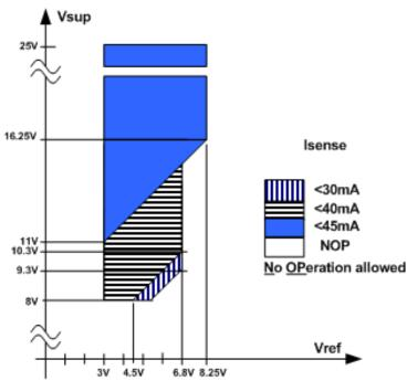
The operating range, and the corresponding maximum Isense, is defined by the Vsup-Vref range as shown in the above graph.
