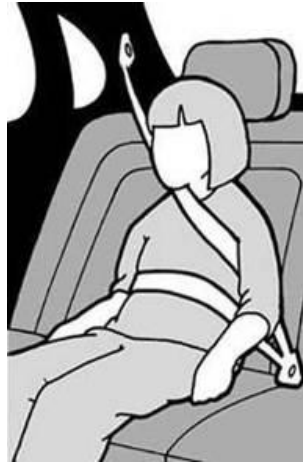
Incorrect belt fit because there is no booster seat
