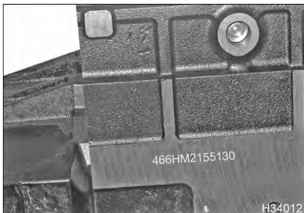
Figure 2 Engine serial number (right side rear)
