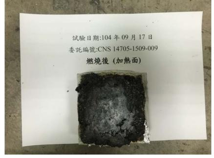
Photo 3, Heating surface, post-test
