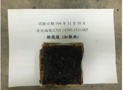
(2) Specimen No. DC315 Fireproof Paint coated on PU Foam (after 1101.34 kGy radiation)
