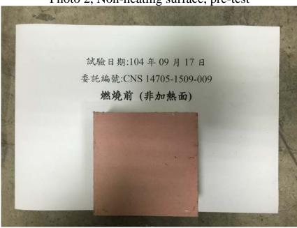
Photo 2, Non-heating surface, pre-test
