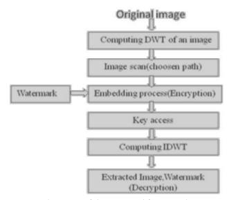
Fig 1. Architecture of the proposed framework DCT of the image been obtained using the formula
