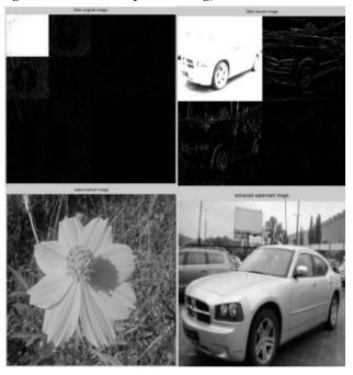
Fig. 4a).DWT of original image (3 bit plane) b).DWT of secret image (3 bit plane) c).Watermarked image d).Extracted watermark image
