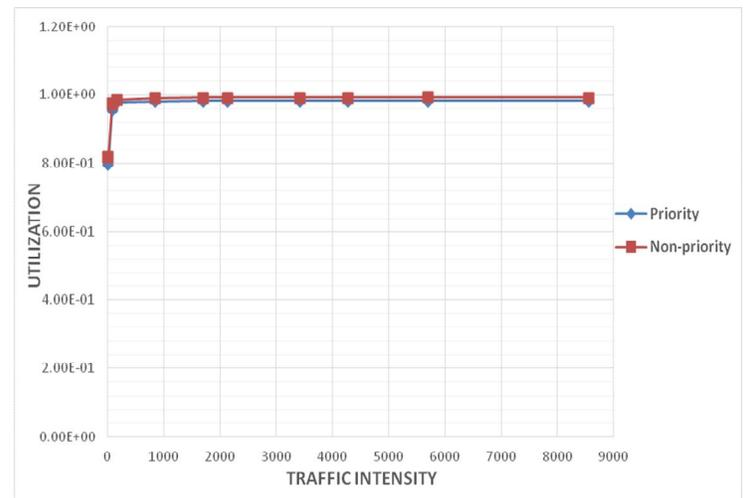
Fig. 4.6 Bandwidth utilization as a function of traffic intensity
