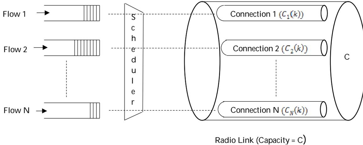
Fig. 3.2: A queuing model of the CDGPS scheme
