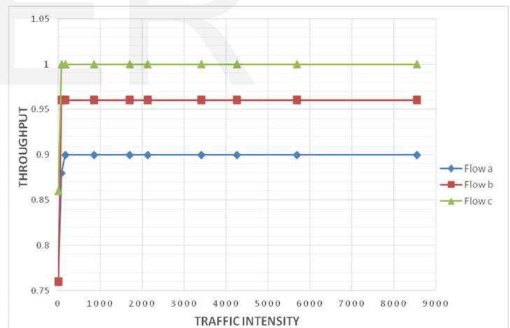
Fig. 4.2: Throughput per flow as a function of traffic intensity
