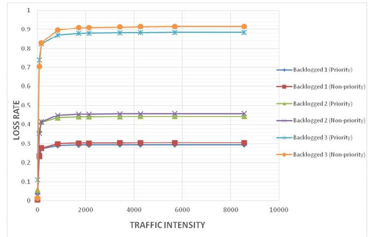
Fig. 4.5 Backlogged flow loss rate as a function of traffic intensity
