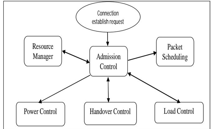
Fig. 2.1: Radio Resource Management Functions Interaction [9]
