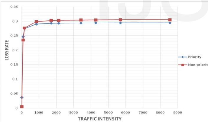
Fig. 4.4: Loss rate as a function of traffic intensity
