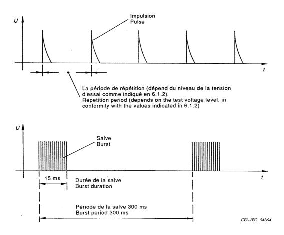
Figure 2 – General graph of a fast transient/burst
