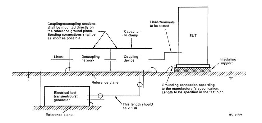
Figure 6 – Block-diagram for electrical fast transient/burst immunity test
