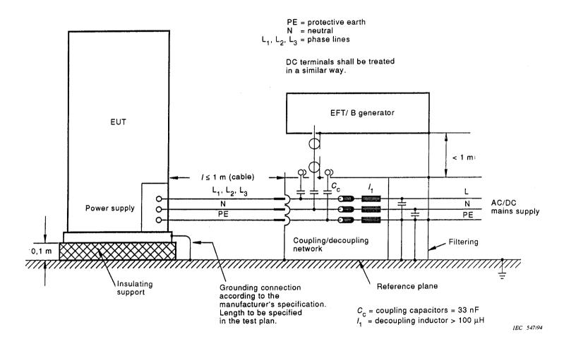
Figure 8 – Example of test set-up for direct coupling of the test voltage to a.c./d.c. power supply ports/terminals for laboratory test purposes
