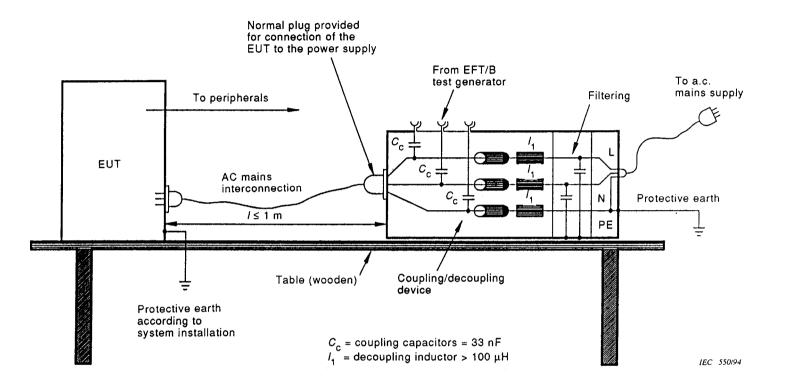
Figure 11 – Example for post-installation test on a.c. mains supply port and protective earth terminals for non-stationary mounted EUT
