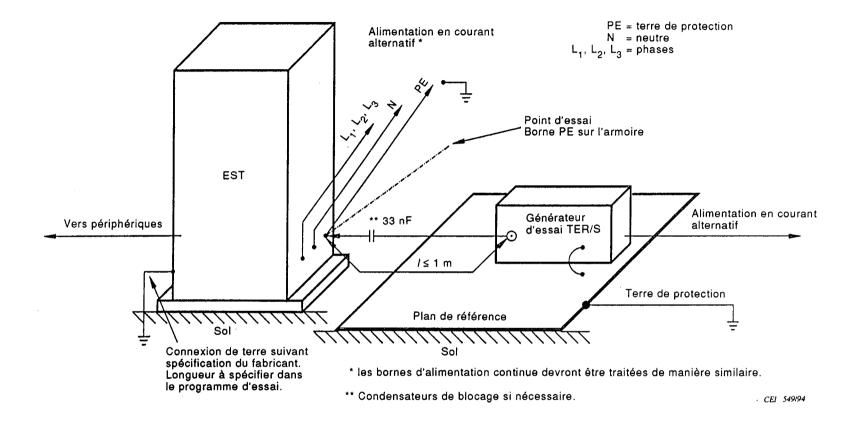
Figure 10 – Example for post-installation test on a.c./d.c. power supply ports and protective earth terminals for stationary, floor-mounted EUT
