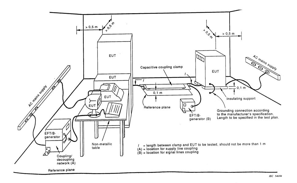
Figure 7 – General test set-up for laboratory type tests
