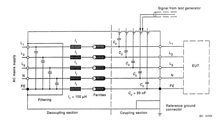
(Example: Construction for three-phase lines, d.c. lines/terminals shall be treated in a similar way.)
