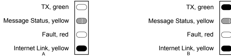
Figure 6. A Registered 7845i Status Display (A) and an Unregistered 7845i Status Display in Normal Operating State
