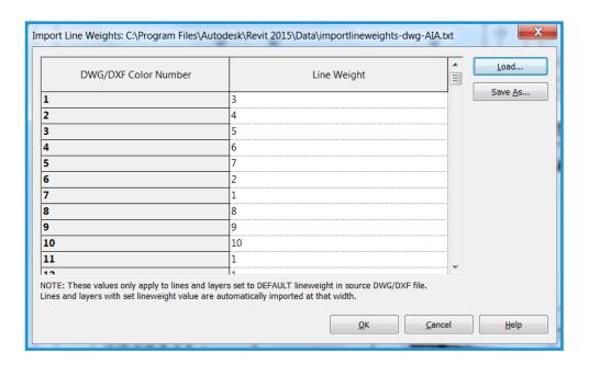
You can review Revit line weight settings going to the Manage tab and selecting Lineweights from the Additional Settings Dropdown on the Settings Panel. Because Revit line weights have different widths at different scales, many imported colors may map to a single line weight
