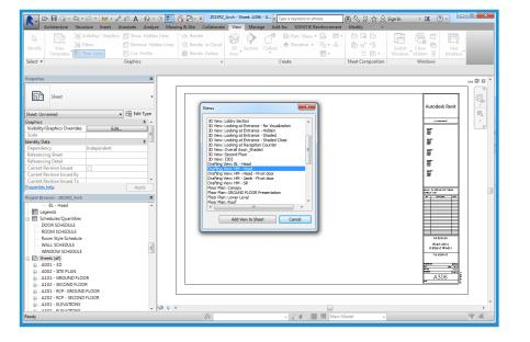
Place drafting views in the same way you would place any view created in Revit. After you have placed the view, the DWG details are part of your Revit set.
