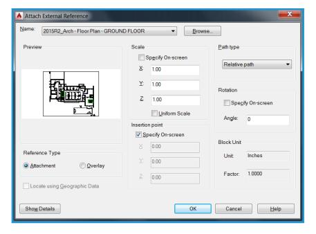
Be sure to use 0,0,0, not Specify On-screen, as the insertion point in AutoCAD. Select Overlay for Reference Type. (Unlike Attachment, an overlaid xref is not included when the host drawing is itself attached or overlaid as an xref in another drawing.)
