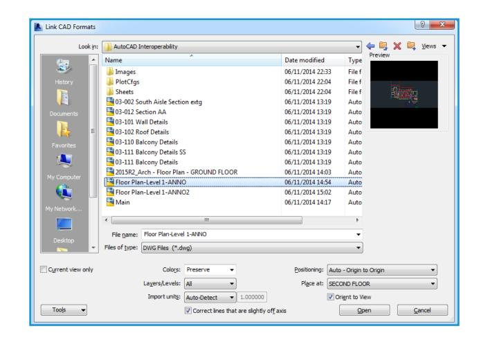
After the file is linked, suppress display of the Revit-generated elements. In AutoCAD, unload the Revit exported file. Return to Revit and click Manage Links from the File menu. Select the linked file, and click Reload.
