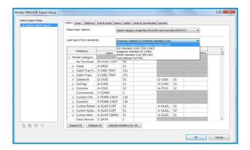
You can incorporate custom office-dependent layering standards into the workflow and apply them to external files. This helps support data consistency within a multi-platform environment.
