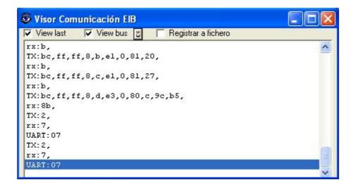
9. Open the External Protocol Communication Viewer window (menu View -> Bus -> External system) and check that there is communication activity, some TX frames and some other ox frames as showed in the figure below. This means that the communication with the BACnet system is ok.
