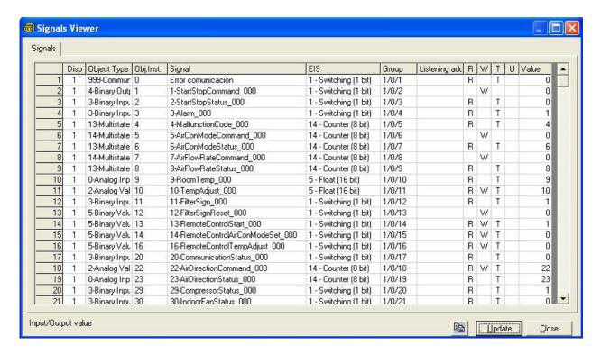
The signals viewer can be used although only one system is connected to the IntesisBox, KNX or BACnet, and is very useful for supervision and test.
