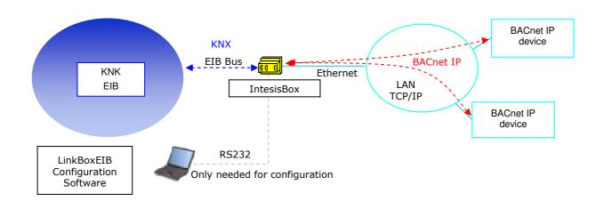
Integration of BACnet and KNX using IntesisBox KNX - BACnet/IP client gateway
