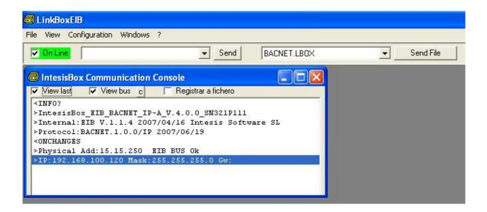
8. Open the EIB Communication Viewer window (menu View -> Bus -> EIB) and check that there is communication activity, some TX frames and some other ox frames. This means that the communication with the KNX system is ok. In case there is no communication activity between IntesisBox and the KNX system check that KNX bus is operative and well connected to the IntesisBox.
