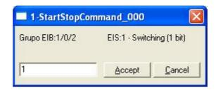
This tool is very useful to test any of the systems connected to the IntesisBox, KNX and *BACnet* without the need to actuate on the real signals.
