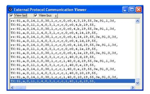
In case there is no response from the BACnet devices to the frames sent by IntesisBox, check that they are operative and reachable from the network connection used by IntesisBox, check the IntesisBox Ethernet interface making pings to its IP address using a PC connected to the same Ethernet network. See details for the communication cable between IntesisBox and BACnet devices in section Connections of this document.
