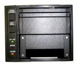
Note: The internal printer uses thermal paper. If not inserted with the correct side up, it will not print. Also thermal ink will fade over time, so this should be avoided for permanent records.
