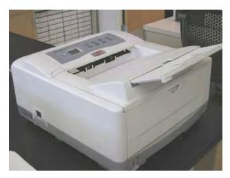
Other compatible printers may be used. Intox has reported that not all printers are compatible, they must be PCL5 or lower. Network printers are an option with the upgraded EC/IR's.
