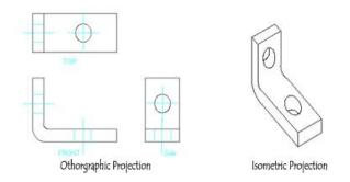
There are rules and conventions to guide the creation of both types of projections. Additionally, either of them can be supplemented with various types of dimensions. Whether sketching or drawing, the goal is the same. The goal is to communicate the necessary detail to the intended audience.
