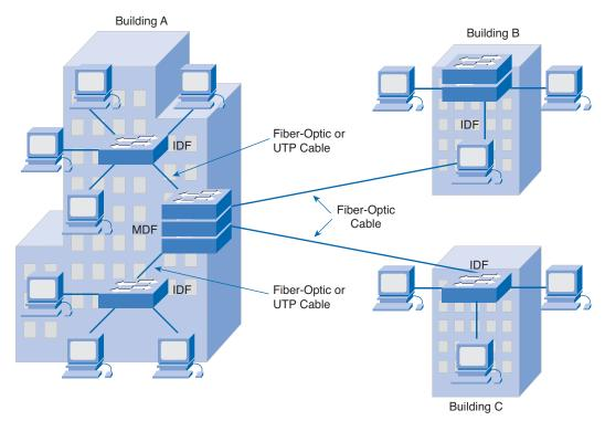
The vertical cabling between the buildings should always be fiber-optic, regardless of distance, to account for the electrical differential between buildings. Inter-building cabling can also be exposed to weather and lightning strikes, which fiber-optic can withstand more easily without damaging equipment connected to it.
