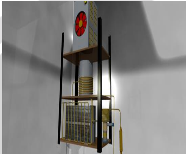
Fig -2: Desert Cooler With VCRS
