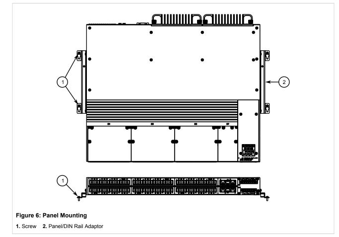
2. Install the supplied screws to secure the adapters to the panel.
