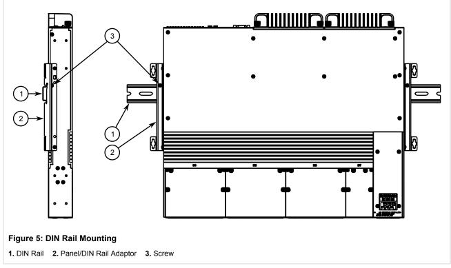
2. Install one of the supplied screws on either side of the device to secure the adapters to the DIN rails.
