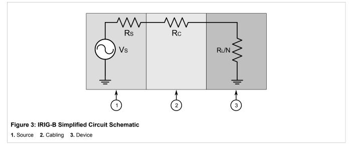
The maximum number of devices (N) that can be connected to the source is determined by checking if the source current (IS) required to drive the connected devices is less than the maximum drive current the source can provide, and verifying that the load voltage (VL) the connected devices see is greater than the minimum required voltage.
