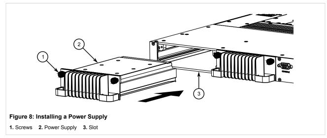
3. Hand-tighten the screws to secure the power supply.
