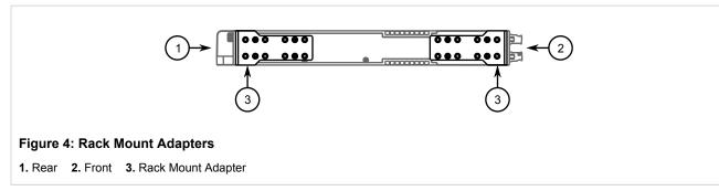
Insert the device into the rack. To make the modules and ports accessible from the front, insert the power supply side of the device first. Reverse the orientation to have the power supplies, management ports and LEDs accessible from the front.
