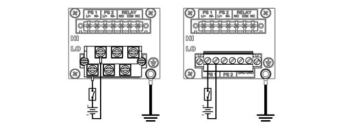
Figure 13: Single Low DC Power Supply
