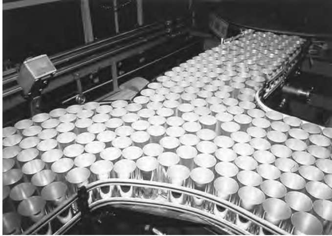
Fig. 1.1 The bodies of beverage cans are alloys 3004 or 3104, making it the largest-volume alloy consumed in the industry. Source: Ref 1.1
