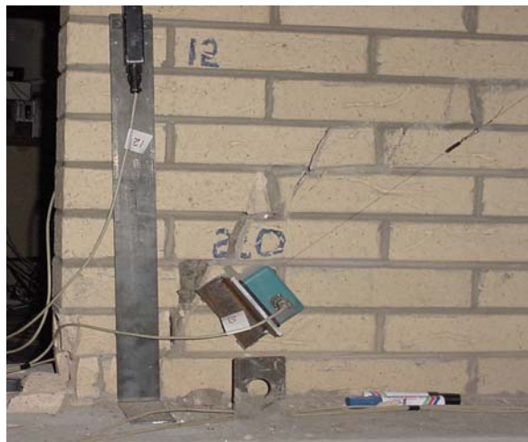
Figure 4.23: Toe crushing of ECRM walls under monotonic loading
