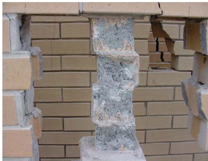
Figure 4.4: Staggering of cores in the test walls
