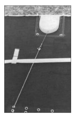
Tie  $3/16'' \ge 6'$  line to one of the shackles and lead the other end through one set of double grommets at center of tramp.
