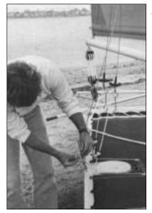
Turn the boat until the wind is blowing from a 45<sup>0</sup> angle to the bow. Ease the traveler out to the lee side and sheet the main in tight. Have your crew sit on the trampoline to keep the mainsheet from uncleating and the boat from tipping. With the main sheeted to lee-
