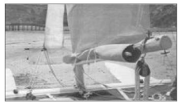
Attach the outhaul car to the aft ring. Starting with the bottom batten, roll the extra sail up and tie with two 2 foot pieces of line using the reef points (grommets) in the sail. Do now tie around boom.
