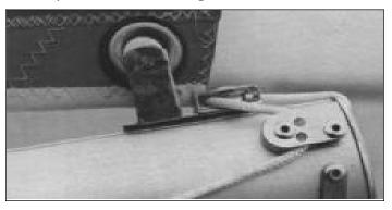
Remove clevis in from outhaul car on aft end of boom and lift boom to aft end of mainsail. Clew ring of sail goes in between sides of outhaul car. Reinsert clevis pin through sail and outhaul car. Install cotter ring in end of clevis pin.
