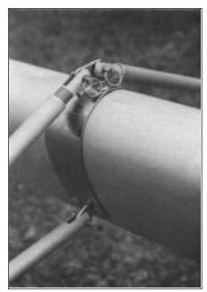
the aft edge of the mast. Cotter rings should be on the bottom. Connect spreader tips with six clevis pins and cotter rings.
