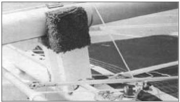
Secure the mast and support to the boat by wrapping the tie down line around the mast twice and down through the trampoline grommets. Store the tiller under a hiking strap or jib lead line to keep it from flapping around. Tie a 3 or 4 foot piece of line to the traveler pad eye, around the tiller crossbar twice, and through the fairlead and cleat. This will keep the rudder castings from swinging. Tie the front end of the mast down making sure to wrap line twice here also.
