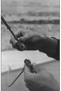
Attach the forestay to the 1/4" shackle holding the bow bridle wires together. After this initial rigging you can leave the forestay turnbuckle preset.
