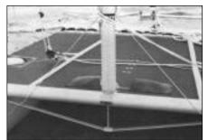
each end to dolphin striker bar on opposite sides of mast. Be sure the jib sheet is lead outside shock cord. This will keep the jib sheet from catching under mast base.
