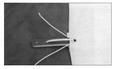
Lead string up through either hole in foam batten or through end cap and down through top grommet and tie an overhand knot (tightly) while pushing batten into sail with thumb.
