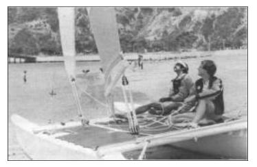
The main traveler should be set a few inches from center with the main sheet snug and the jib sheet slightly looser than used when going to weather. This will allow the distance between the main and the jib to increase. Both sails should be sheeted in so that both the leeward and windward telltales are streaming back.
