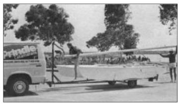
Lace the forestay through the back lace lines 2 or 3 times. Store trapeze dogbones under trampoline to keep them from banging around. You may wish to tie the wires up off the front crossbar to keep them from rubbing on a long trip with a line over the mast.
