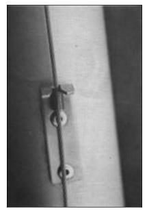
When the sail reaches the top of mast, you must secure the second metal stop on the halyard wire into the halvard lock on the mast. DO this by leading wire between teeth on lock and pulling down on sail to put tension on the metal stop. The other stop, further down on the halvard wire,
