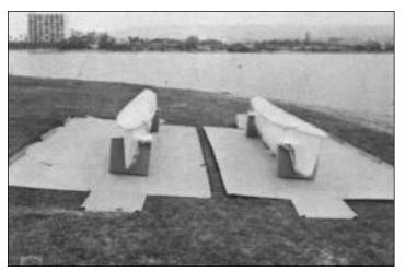
Open the hull containers. Leave the hulls standing on the cardboard supports.
