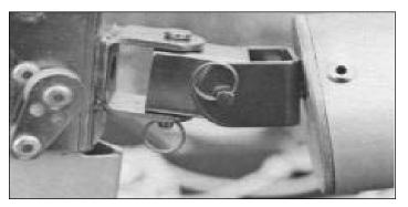
Remove clevis pin from gooseneck assembly attached to forward end of boom. Connect boom to the bracket on the mast using this clevis pin and cotter ring.
