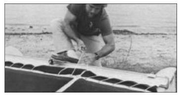
Stand at the back of the boat and tighten lines by bracing your foot against the rear crossbar for leverage. Pull as tight as possible. Tie off lines under trampoline. Do not trim excess line as this leaves something to hold when retightening tramp.
