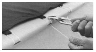
Tighten each side by using a pair of pliers or vice grips. Start tightening from the front and move to the rear. Be sure to get trampoline centered on boat by lining up the grommet nearest the front crossbar with the center of the mast step. Trim and burn excess line. Save for use later.
