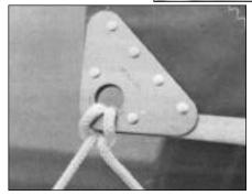
shackle pin. Make sure that these lines are not twisted. Pull up slack from line leading between the jib sheet blocks and trampoline.
