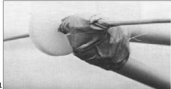
**DANGER! SPECIAL ATTENTION:** Be sure all spreader fittings are securely attached. The mast will break if the diamond wires come loose. The mast is not covered under warranty for breakage due to improper tun ing, assembly or maintenance.
