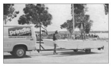
Attach mast hinge to the mast. With one person on the trampoline, push the mast forward and disconnect the forestay shackle. DO NOT undo the turnbuckle. Rig shackle so it holds the two bow bridle wires together. Check in back of boat to make sure you will not be lowering the mast onto a person, car, or power line.
