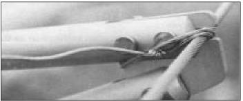
Place the diamond wire in the slot in the spreader tip with the nylon roller above the spreaders. Using one of the 9" pieces of seizing wire, seize the diamond wires in place so they cannot come loose. You must wrap the tips with duct, sail or electrician's tape to protect your jib from chafing.
