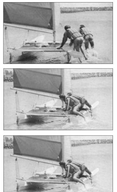
Push the boat off at a 45 to 60 degree angle to the wind until it floats, jump on and sheet in the jib (only) tight. (Do not sheet in the main yet.) This will pull you out at a good angle until you can safely drop your rudders. As soon as water is deep enough, drop and lock both rudders, bring traveler to center and sheet in main. You're off!
