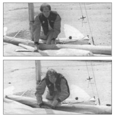
Insert the rolled jib and continue rolling.
