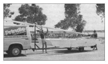
While the second person holds the mast, remove the hinge pin and walk the mast forward until you can place it in the front mast
