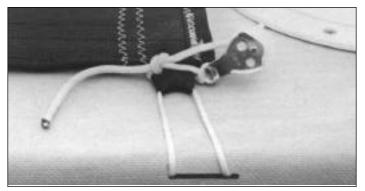
Tie the block onto the side trampoline tab using a square knot. Use tab just forward of hatch for single trapeze and tabs just forward and aft of hatch for double trapeze.
