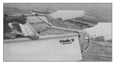
To raise the rudder, grab handle at end of tiller and pull until desired height of rudder is achieved.
