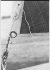
Lead jib downhaul line around shackle pin and cleat downhaul line snugly into cleat on jib tack.
