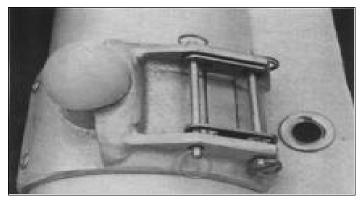
This photo shows the mast step and hinge. Store hinge components as shown when not in use.
