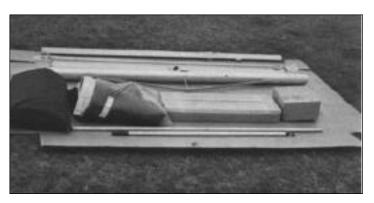
boom battens rear crossbar front crossbar sails trampoline rudder box rigging box tiller crossbar tiller extension
