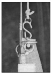
Hoist jib up, closing sipper as you do until "S" hook just passes ring.
