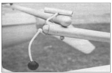
In operation if the rudder is pulled up too far, the head of the rudder blade will hit the washers at the top of the casting. This could chip your rudder blade. To prevent this, tie a knot in pull down line about 3" from ball. Adjust position of know so that the raised rudder stops just short of hitting the washers.
