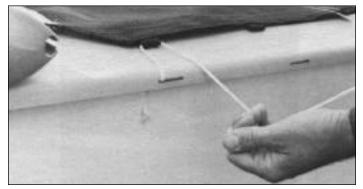
Tie a figure eight knot in the end of side lacing line  $(1/8" \times 11')$  and begin lacing side of trampoline beginning at forward slot. Lace line up through deck, through forward loop and back down through deck. Proceed aft and tie off end. Follow same procedure for other side of trampoline.
