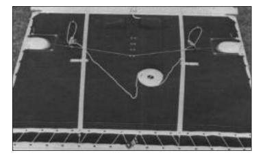
Hiking straps on trampoline are adjustable for personal comfort. People with long legs use the inboard look. Tie off onto a grommet at rear of tramp.
