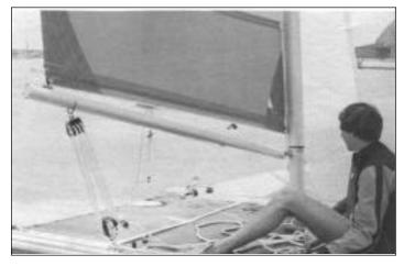
The main traveler should be centered with the main and jib sheets in snug. Be careful not to pull the sails in too tight. If the main is oversheeted (too tight), the mainsail will be too flat and the boat will not move very fast.
