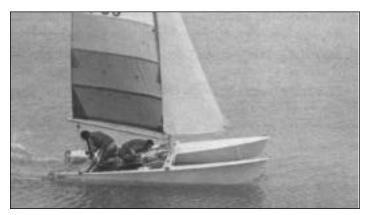
The skipper should now move aft, into the center, and swing the hiking stick to the new side. Do not straighten the rudders out. If you do, you will find yourself into "irons" (boat pointing directly into wind making no headway).
