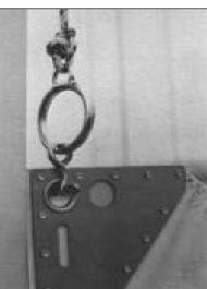
Attach the twisted shackle to the head of the mainsail and place forward edge of sail into curf of mast.
