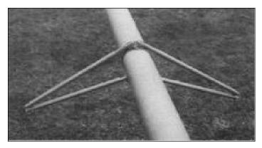
The adjustable forward bar can be lengthened or shortened to adjust the amount of "sweep back" the spreaders have. The more the spreaders are "swept back", the smoother the mast bend will be, even with tight diamond wires. However the more "swept back" the spreaders are the more they will get in the way of the jib while sailing. There is no "right" or "wrong" in the amount of "sweep back" - just personal preference. Be sure both sides are adjusted to the same length.
