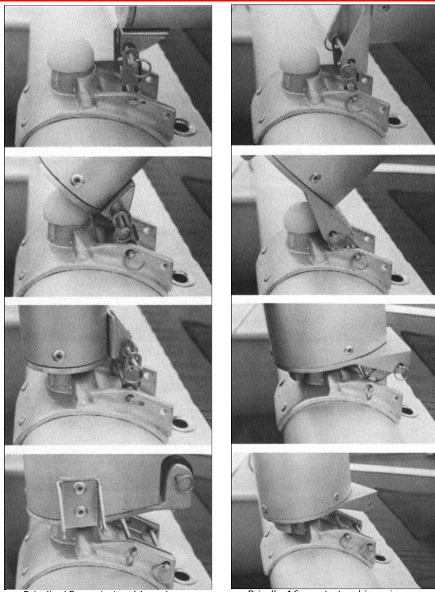
Prindle 15 mast step hinge in use
