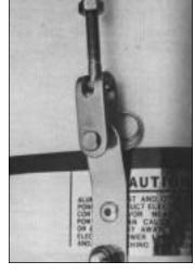
The turnbuckle on the diamond wire is attached to the lower fitting on the mast. The two separate turnbuckle studs should be started into the turnbuckle at the same time.
