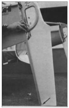
edge flush against the transom. Adjust the lock bolt so that the forward bottom edge of the rudder is about 1/2" aft of the forward edge of the batten. (Pull rudder back lightly to pull out any slop.) 1/2" aft is a good starting point, further adjustment may be necessary for personal preference.
