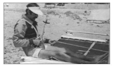
Sit on the side of the hull just forward of the shroud. Pull the dog bone down and hook the uppermost ring onto the harness hook.
