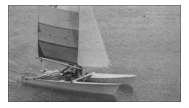
When the bows are pointing into the wind, release the main sheet 1 or 2 feet. Leave the jib cleated.
