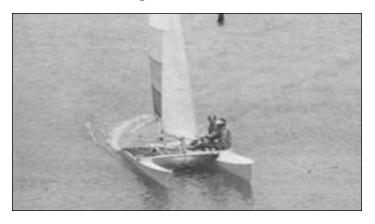
Make a smooth turn to windward using about one half the amount of rudder throw. Turning the rudders too sharply will stall the boat and bring it to an abrupt stop.
