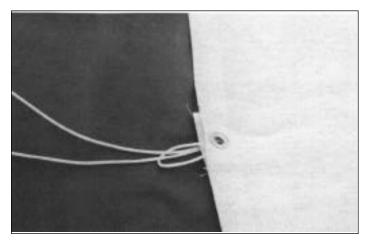
Fold batten string in half and loop through batten grommet on leech of sail.
