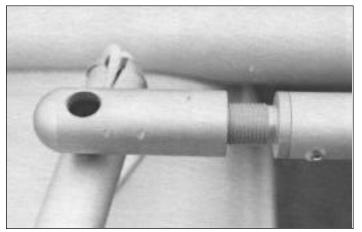
trailing edges is 75.5"; unscrew the tiller adjuster 4 or 5 complete turns and measure again. Keep adjusting until the measurements are the same. You can achieve accuracy up to 1/32" of an inch, but 1/8" is good.
