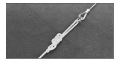
Attach jib blocks to thimble at end of jib bridle wire (not shackle) using 3/16" shackle. Be sure the jaws of cleat face inboard. Thread 5/16" x 33' jib sheet line by tying off one end to jib block with bowline. Thread through small jib clew blocks, through cleat on jib
