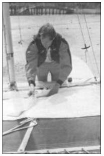
Roll tightly without any folds. If it is windy, put the jib under the hiking strap to keep it from blowing a way while you lower the main.
