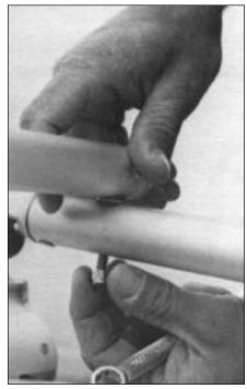
and tiller arm. Insert 1/4" bolt through hole in tiller arm and put lock nut on end. Make sure lines inside tiller go on either side of bolt, do not cross them. Do not put the nut on the bolt at adjuster end of crossbar until the rudders have been aligned (instructions later).
