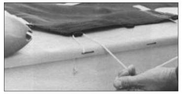
hole in the deck. Put some silicone sealant on your forefinger and reach through the hatch to put the sealant on the bolt where it enters the hull. Attach lock nut and flat washer to bolt inside hull using 1/2" box-end wrench. If you cannot reach the bolt, tape the nut to the wrench. Thread nut snugly to hull. Do not tighten until all bolts are snug.
