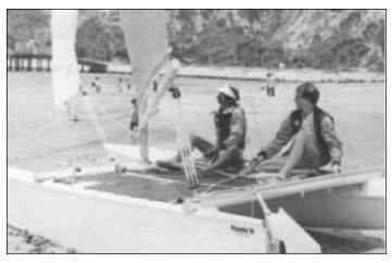
Let the main traveler all the way out to the end of the crossbar and sheet the main loosely. Do not let the main out far enough to rub against the shrouds if at all possible. Trim the jib sheet loosely trying to keep the windward and leeward tell-tales streaming back.
