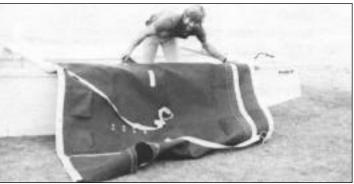
From the port hull, insert forward and rear edges of trampoline in curfs on crossbars. The rear edge has two rows of grommets.
