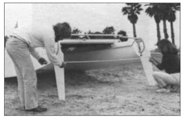
Measure from the centerline of the front edge of one rudder blade (22" up) to the centerline of the front edge of the other blade. Do the same with the trailing edges.
