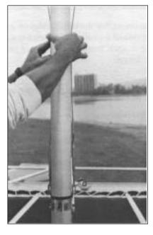
Prindle 18: Adjusting the tension of the diamond wires should be done with care. Before the sails are hoisted, but after the mast has been stepped; adjust both diamond wires to the same tightness. If one is looser than the other your mast will bend more on one tack than the other.
