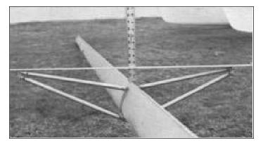
To measure the amount of "sweep back" in the spreaders, lay a batten or yard stick from tip to tip. Then measure the distance from the curf on the mast to the batten. About 1.5" "sweep back" is considered normal.
