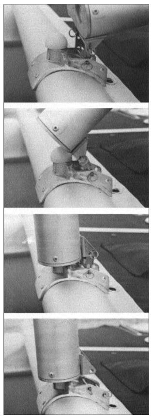
Prindle 18 mast step hinge in use
