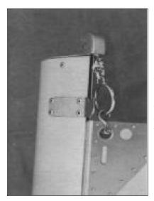
When the sail reaches the top of the mast, you must lock the ring on the halyard line to the hook at the head of the mast. To do this, pull halyard until the ring is above the hook.
