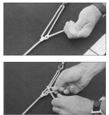
Using a truckers hitch, tie the line to the 3/16" shackle on opposite jib bridle wire. Pull line as tight as possible and tie off using a row of half hitches.
