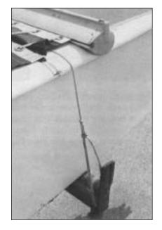
Place the boat on the trailer. Tie the boat down using at least 1/4" nylon or dacron line. DO NOT TIE ANYTHING TO THE DOL-PHIN STRIKER OR ROD. Remove the rudder blades from castings. Be sure they are marked port or starboard so you don not have to retune them the next time you go sailing.
