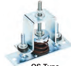
OS Type Steel Spring Isolator Restraints 1", 2", & 3" Deflection Pages 273 & 274
