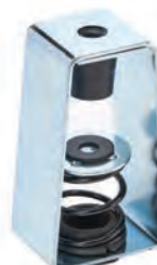
HH30SCS Type Deflection Combination Hanger 15° Tilt Spring & Neoprene w/ Seismic Cushion Stop 1 1/2" & 2 1/2" Deflection Pages 289 & 290
