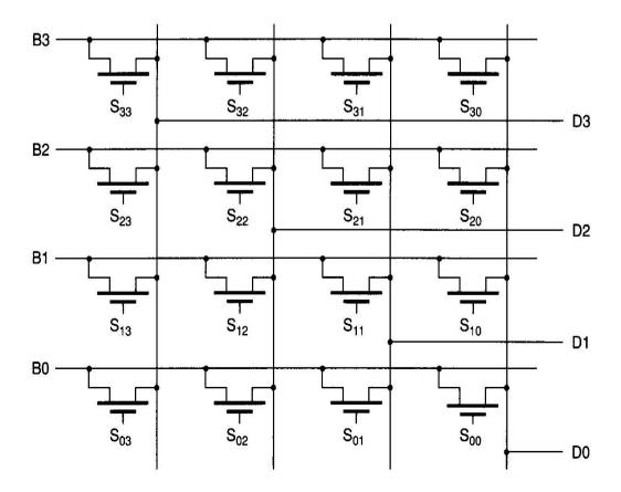
Fig. Barrel shifter (4 control lines S0-S3)
