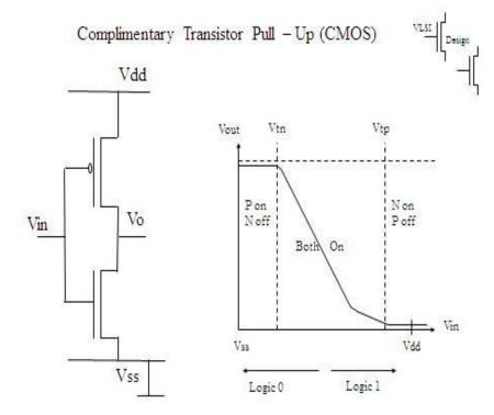
Figure. Static CMOS Inverter
