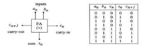
Figure 5.45 Full adder operation
