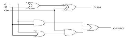
Figure.4.1 Gate schematic for conventional full adder
