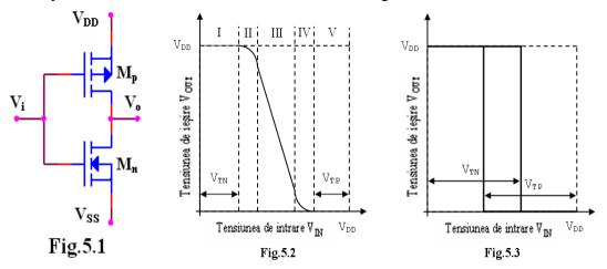
Figure 14. VTC of CMOS Inverter
