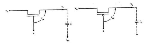
Figure. n and p pass transistors.
