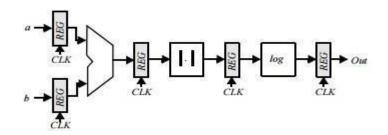
Figure 3.15 Pipelined version
