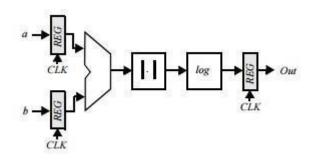
Figure 3.14 Non pipelined version
