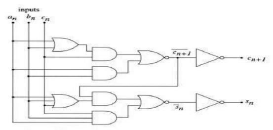
Figure 5.46 Full adder circuit using AOI structuring
