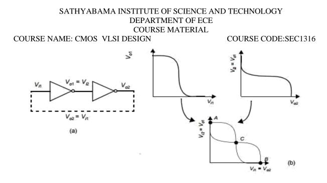
Figure 3.3 VTC of Flip-Flop
