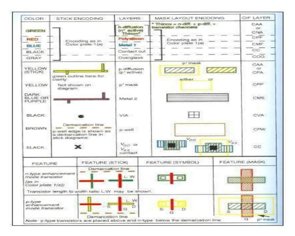
Figure. CMOS encodings.
