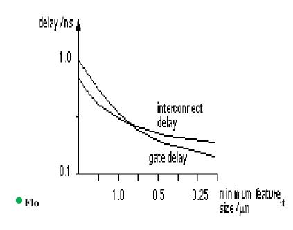
• FIGURE 16.3 Interconnect and gate delays. As feature sizes decrease, both average interconnect delay and average gate delay decrease—but at different rates. This is because interconnect capacitance tends to a limit that is independent of scaling. Interconnect delay now
