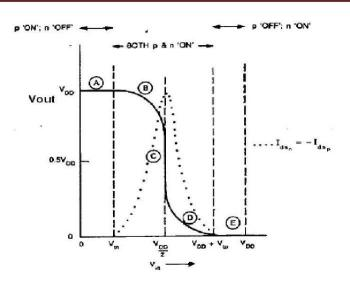
Figure.18 DC Characteristics of CMOS Inverter
