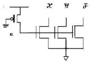
Figure: Multi drain logic
