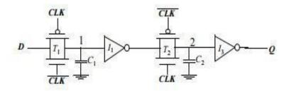
Figure 3.10 Dynamic edge triggered register
