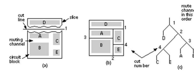
• Defining the channel routing order for a slicing floorplan using a slicing tree.
