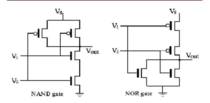
Figure. Schematic diagrams of nand and nor gate
