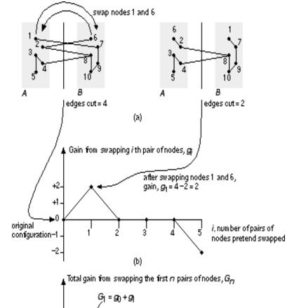
• FIGURE 15.9 Partitioning a graph using the Kernighan–Lin algorithm.
