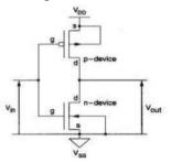
Figure 15. Logic diagram of CMOS Inverter
