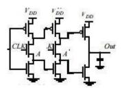
Figure 3.19 Positive edge-triggered D-Flip-Flop using split-output latches
