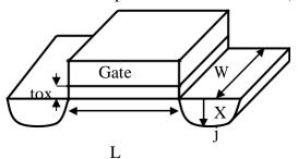
Figure 13. MOSFET Scaling
