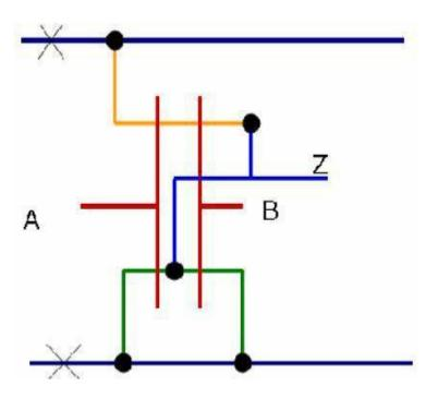
Figure. Stick diagram of NOR gate
