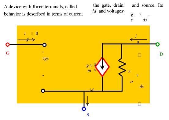
Figure 26. Small signal model of MOS transistor
