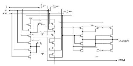
Figure 4.2 Transistor level schematic for conventional full adder
