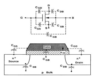
Figure 2.9: MOSFET Capacitance Model
