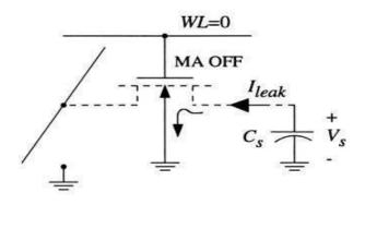
$$t_H \approx \frac{C_s}{I_{leak}} \left( V_{max} - V_1 \right)$$
