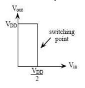
Figure.16 Ideal Characteristics of an Inverter.
