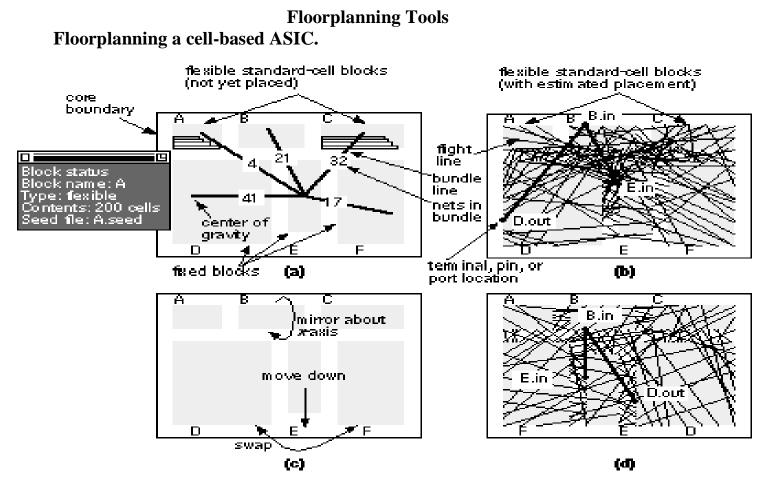
(a) Initial floorplan generated by the floorplanning tool. Two of the blocks are flexible (A and C) and contain rows of standard cells (unplaced). A pop-up window shows the status of block A.
