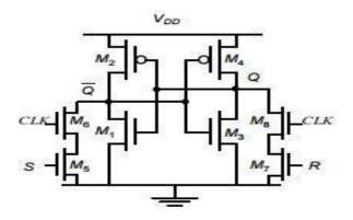
Figure 3.6 CMOS clocked SR FLIPFLOP
