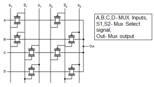
4:1 MUX using transmission gate
