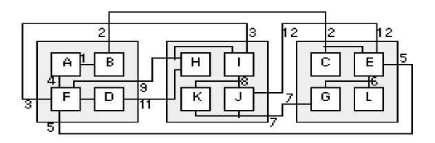
• A constructed partition using logic cell C as a seed. It is difficult to get from this local minimum, with seven external connections (2, 3, 5, 7, 9, 11, 12), to the optimum solution of b.
