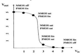
Figure.17 Actual Characteristics of an Inverter.
