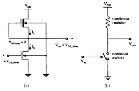
Drawbacks of the enhancement load inverter can be overcome by using depletion load inverter. Compared to enhancement load inverter, depletion load inverter requires few more fabrication steps for channel implant to adjust the threshold voltage of load.
