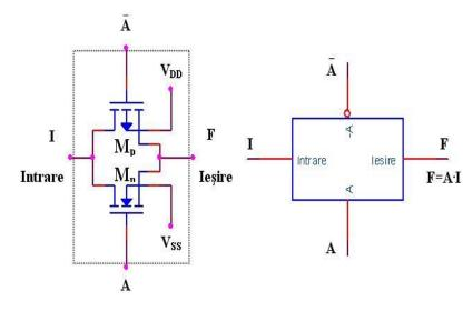
The circuit acts like a switch, the logic variable A being the control input. When the control input A is in logic "1" and  $\overline{A}$  in logic "0" the transmission gate is open, and between the input and output appears a small resistance which lets the current flow in any direction.
