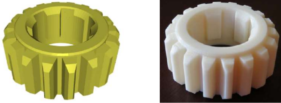
Fig. 7: 3D print of a gear model.
