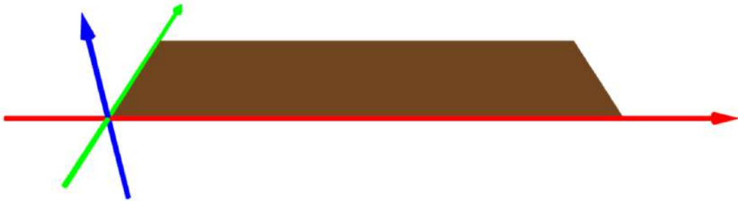
Fig. 18: Copper rectangle of dimensions a \times b with a = 3, b = 1 , as a thin 3D solid.
