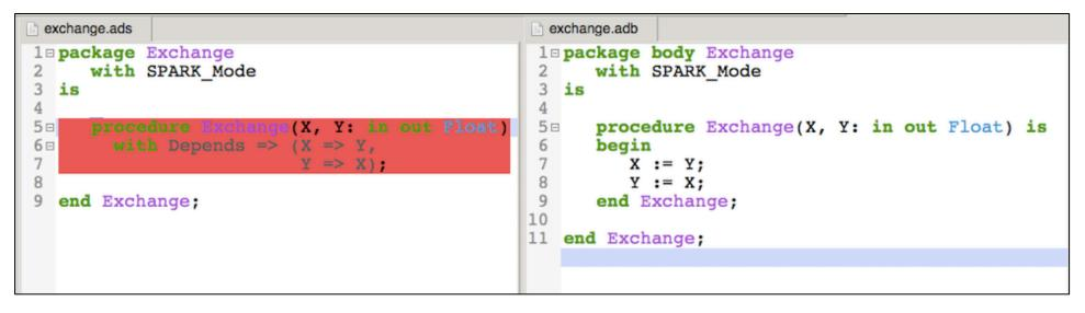
warning: unused initial value of "X" warning: missing dependency "null => X" warning: missing dependency "Y => Y" warning: incorrect dependency "Y => X"
