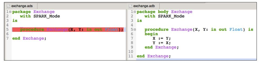
Phase 1 of 2: frame condition computation ... Phase 2 of 2: analysis of data and information flow ... exchange.ads:5:23: warning: unused initial value of "X"
