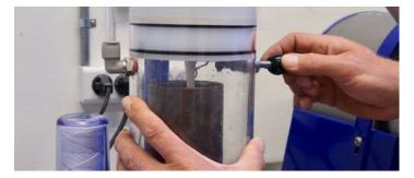
3 Slowly pour the investment down the side of the flask, avoiding the pattern tree. A smooth pour is less likely to trap bubbles. Use a vacuum chamber to extract any bubbles from the flask. Allow the investment to harden and dry.
