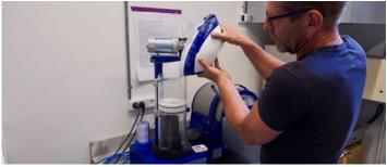
2 Mix investment powder and cold distilled water according to manufacturer's instructions. Adding slightly less water to the mixture will usually increase investment strength, although viscosity will also increase (more difficult to degas). Mix on slow speed until the powder is completely wet.
