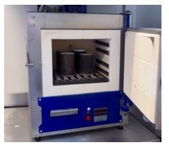
Place flasks in a well ventilated burnout oven.
