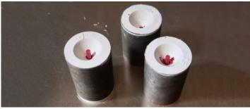
4 Carefully remove rubber sprue base from the flask and allow it to set in a vibration-free environment for 2-6 hours.
