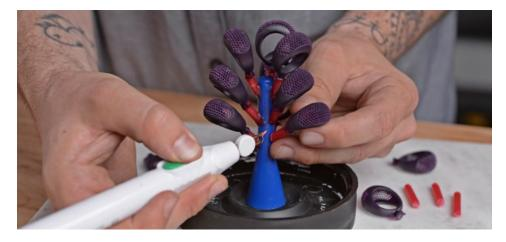
Arrange thicker parts at the bottom and thinner parts at the top of the tree. 3D printed parts may require slightly more space between parts than a traditional wax tree. If you are casting large "thin-shelled" parts, make sure to fill any drain holes with wax to prevent any investment material from entering the print.
