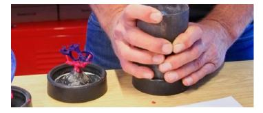
1 Attach a casting flask to the sprue base. If the flask is perforated, wrap it with clear packing tape to contain the investment.
