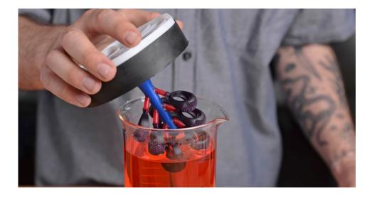
A <u>wax heat pen</u> makes it easier to join resin patterns to the wax sprue tree.
