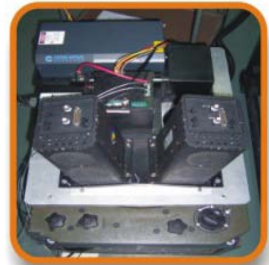
Airborne pushbroom imaging spectrometer (0.45 \mu\text{m} -2.5 \mu\text{m} )
