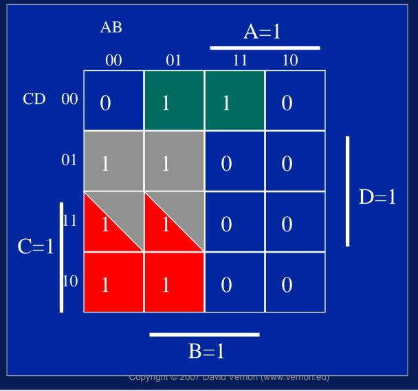
$f2 = B.\underline{C}.\underline{D} + \underline{A}.C + \underline{A}.D$
