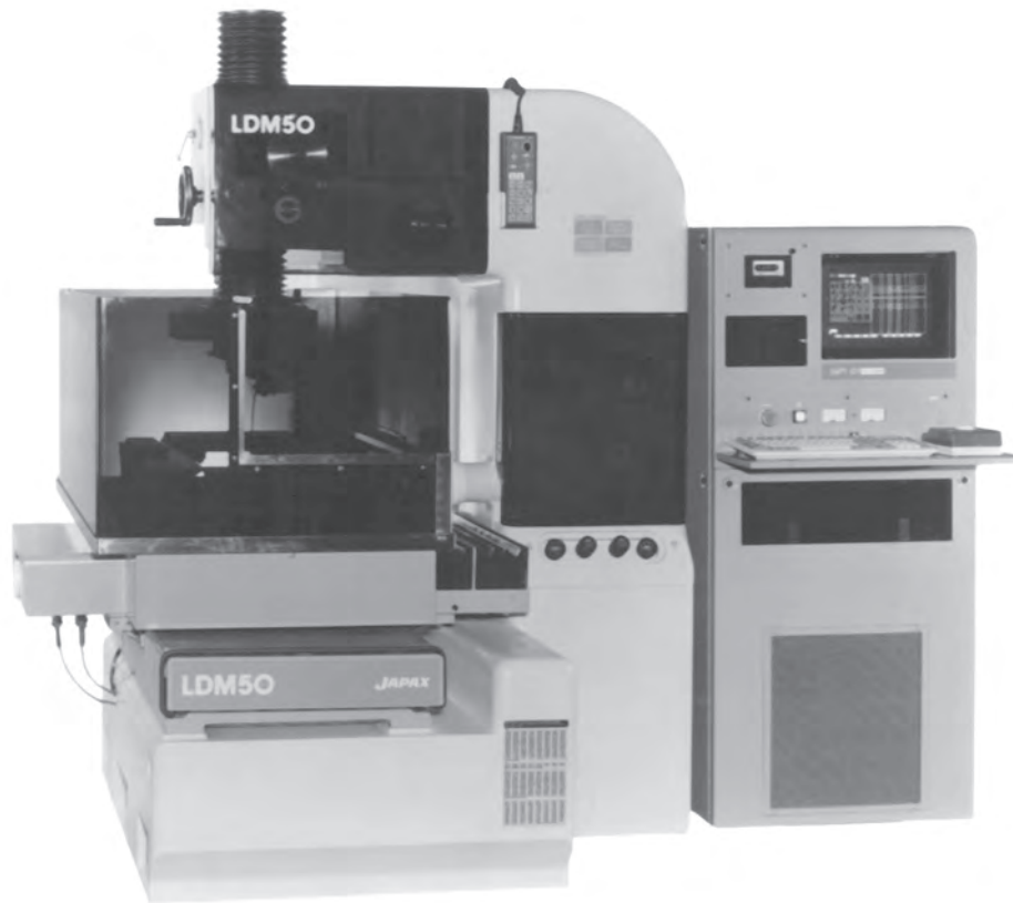
FIGURE 1.9 A CNC-controlled wire cutting EDM machine. (Photo courtesy of James V. Valentino.)
