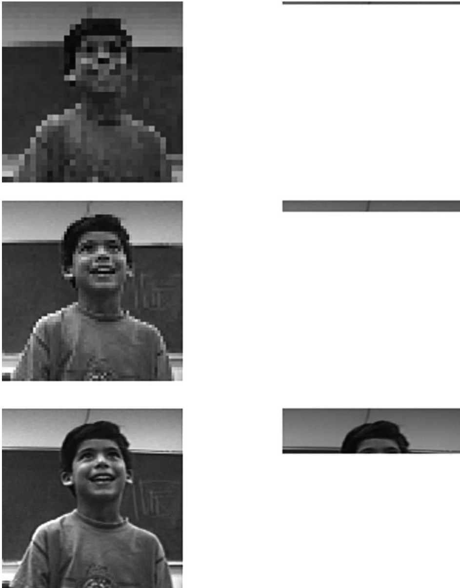
FIGURE 7. 4 Comparison between the received image using progressive transmission and using the standard raster scan order.
