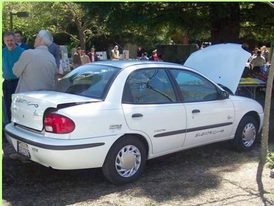
1998 Solectria Force: 84 mile range, NiMH batteries
