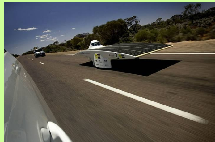
DIT Nuna: drove 1877 miles averaging 55.97 MPH on solar power in 2007, LiPo batteries
