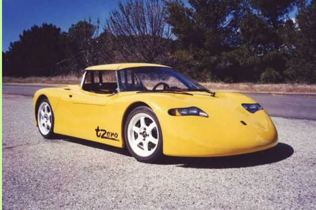
AC Propulsion tZero: drove 302 miles on a single charge at 60 MPH in 2003, Lithium Ion batteries
