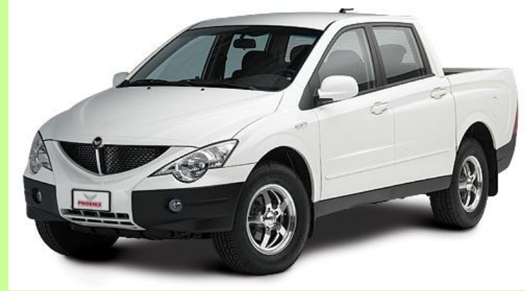
Phoenix Motorcars SUT: charged 50 times in 10 minutes with no degradation in 2007; 130 mile range
