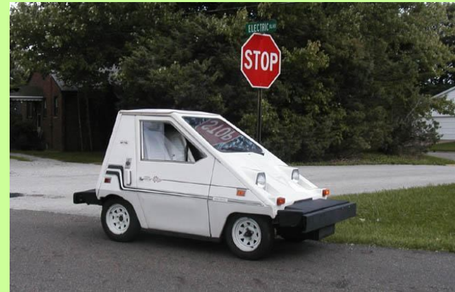
1980 Commuter Vehicles CommutaCar: 30 MPH, 40 mile range, PbA batteries
