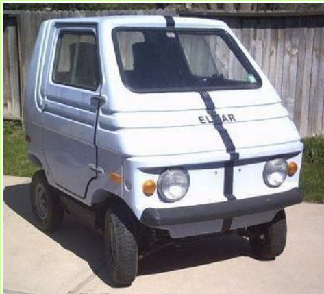
1974 Zagato Elcar: 35 MPH, 35 mile range, PbA batteries
