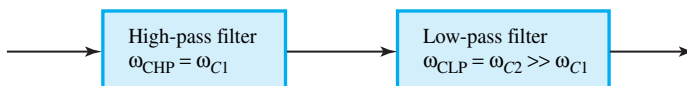
Figure E3.6.3 Bandpass filter through cascade connection of high-pass and low-pass filters.
